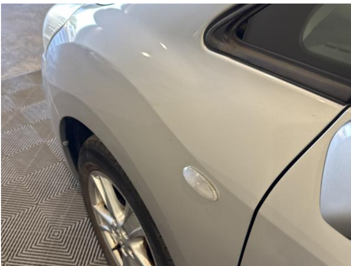
7: Wing nsf Poor Previous Repair Rippled UpTo 30%
