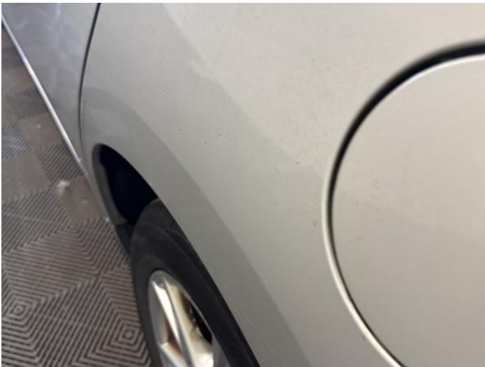
11: Qtr Panel nsr Dented Between 10mm + 30mm
