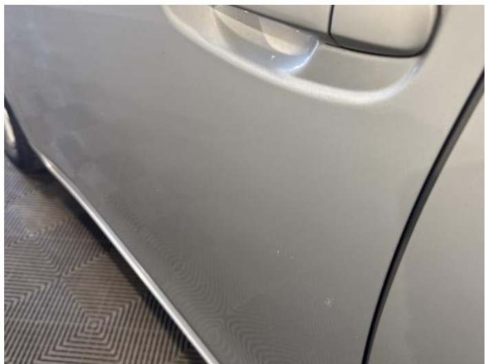
8: Door nsf Poor Previous Repair Poor Paint
