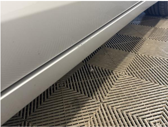
19: Sill Panel Trim os Scratched (Painted) Over 25mm Thru Paint
