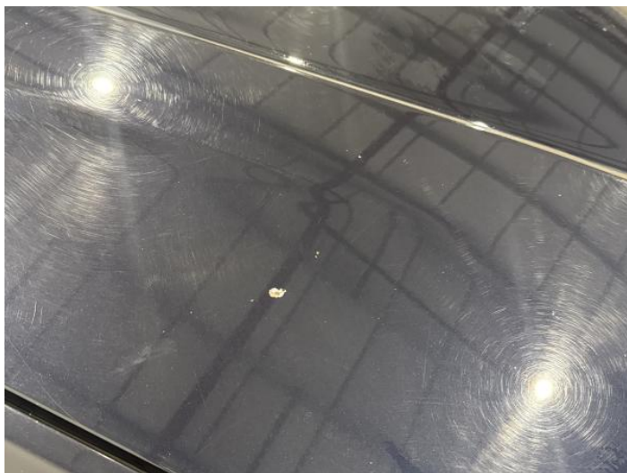
1: Bonnet Chipped Over 5mm
