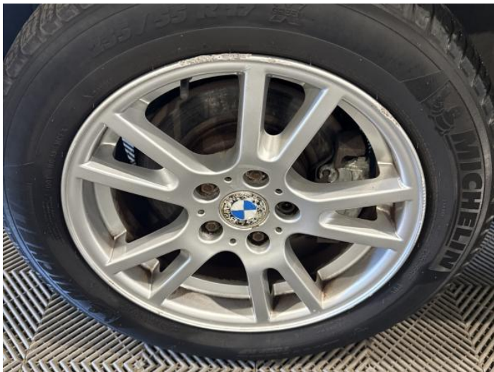
3: Wheel nsf Scratched Over 50mm
