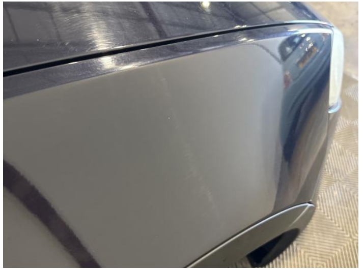
18: Wing osf Scratched UpTo 25mm Thru Paint
