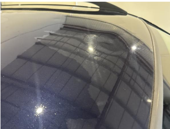
19: Roof Dented Over 30mm
