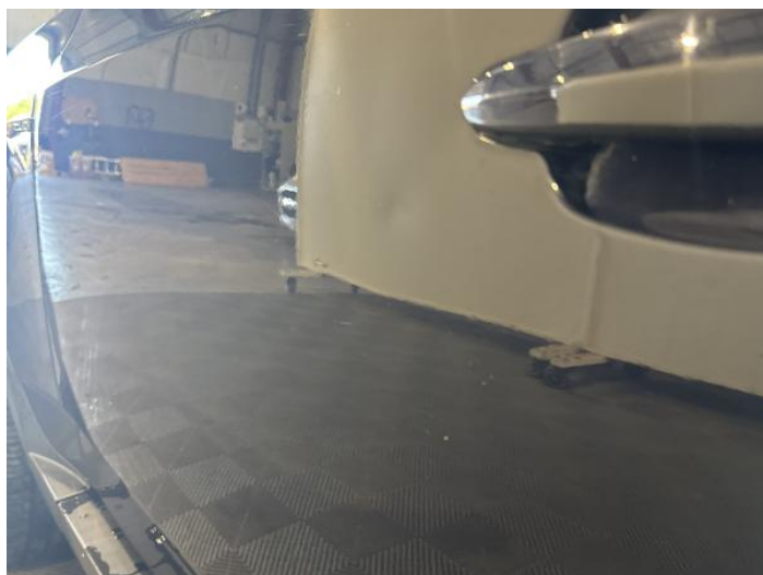
6: Door nsf Dented With Paint Damage
