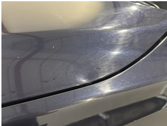
4: Bonnet Dented With Paint Damage
