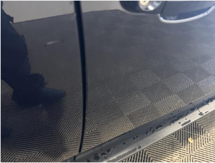
15: Door osf Chipped Edge Chip
