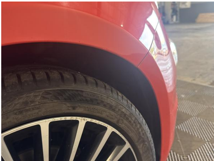
15: Wing osf Scratched UpTo 25mm Thru Paint
