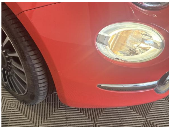
2: Bumper Front Scratched 25 to 100mm Thru Paint
