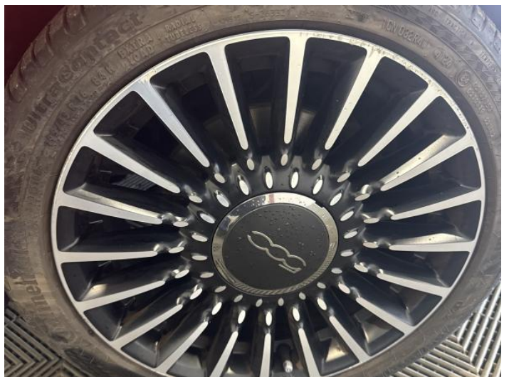
14: Wheel osf Scratched Over 50mm
