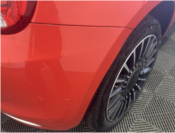
9: Bumper Rear Scratched 25 to 100mm Thru Paint
