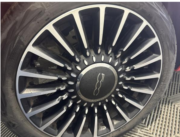
13: Wheel osr Scratched Over 50mm
