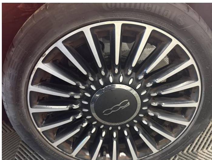
8: Wheel nsr Scratched Over 50mm
