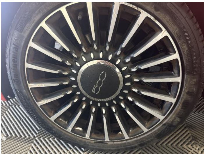
3: Wheel nsf Scratched Over 50mm
