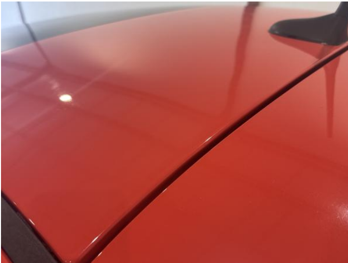
11: Roof Dented Hail - Moderate
