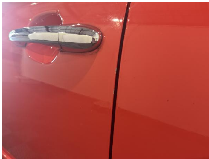
6: Door nsf Chipped Edge Chip
