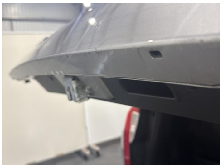
14: Tailgate Trim Panel Scratched (Painted) Over 25mm Thru Paint
