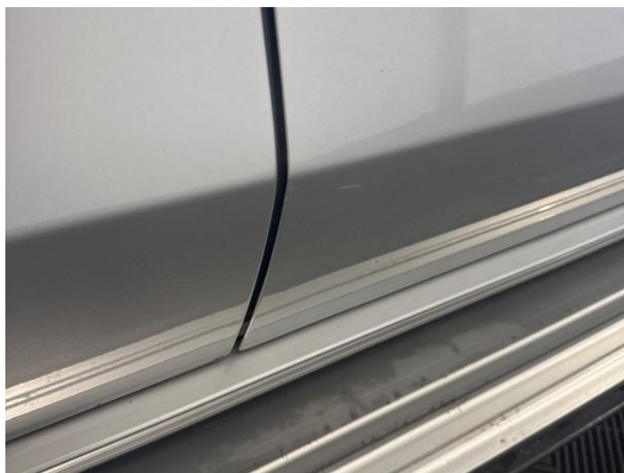
18: Door osf Scratched UpTo 25mm Thru Paint
