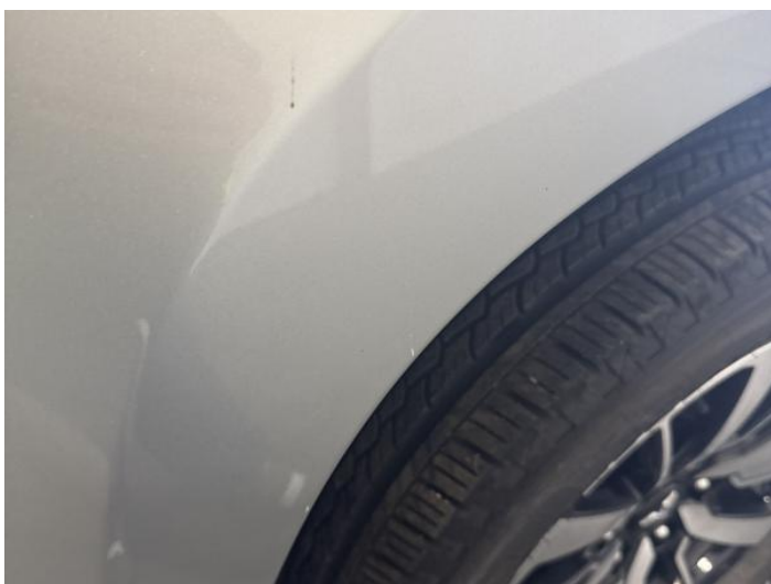
19: Wing osf Scratched UpTo 25mm Thru Paint
