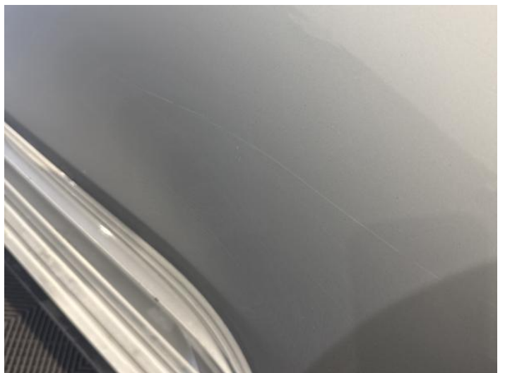
8: Door nsr Scratched Over 25mm Thru Paint
