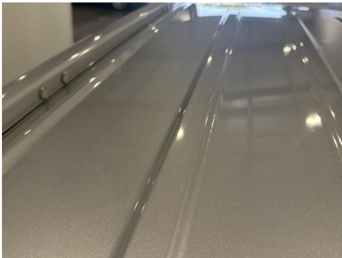
15: Roof Dented Between 10mm + 30mm
