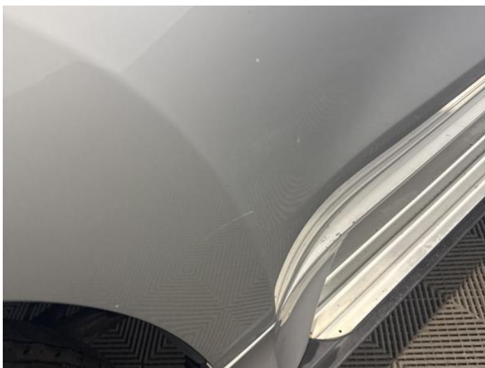
17: Door osr Scratched Over 25mm Thru Paint
