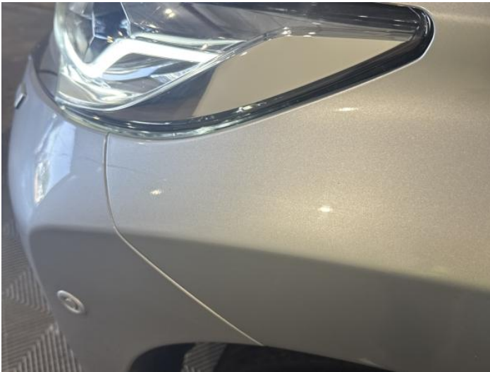
5: Wing nsf Scratched UpTo 25mm Thru Paint
