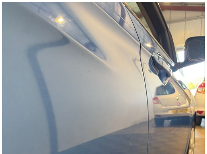
8: Door osr Dented With Paint Damage
