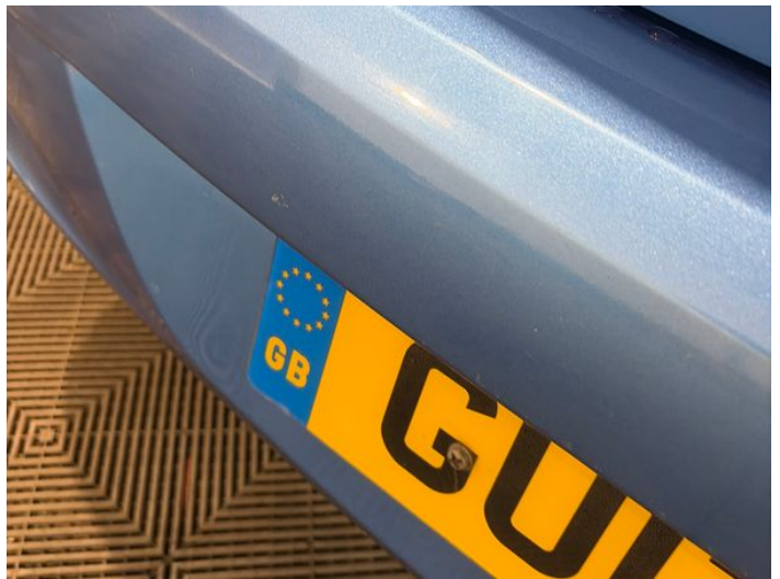
6: Bumper Rear Chipped 1 To 5
