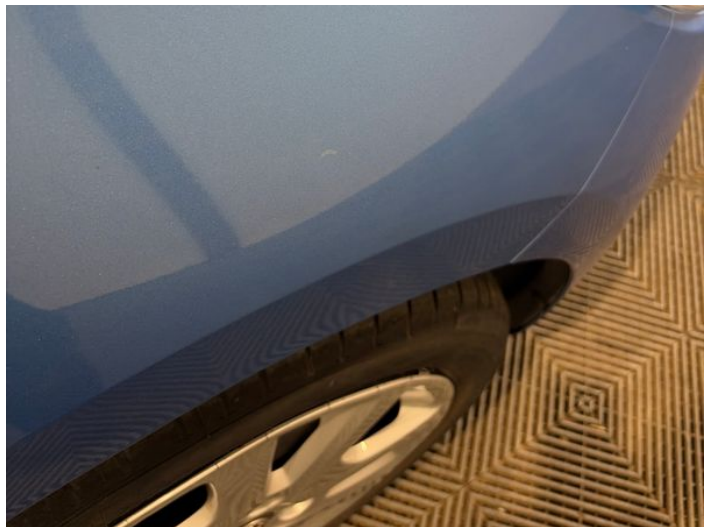
10: Wing osf Scratched UpTo 25mm Thru Paint
