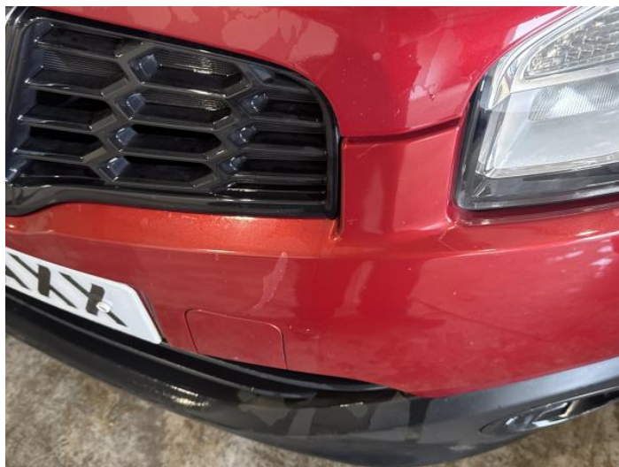
2: Bumper Front Poor Previous Repair Paint Flake
