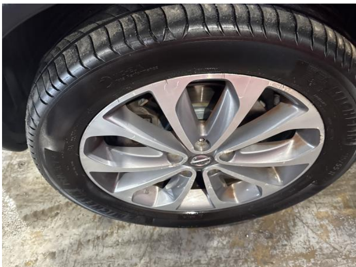
3: Wheel nsf Scratched Over 50mm
