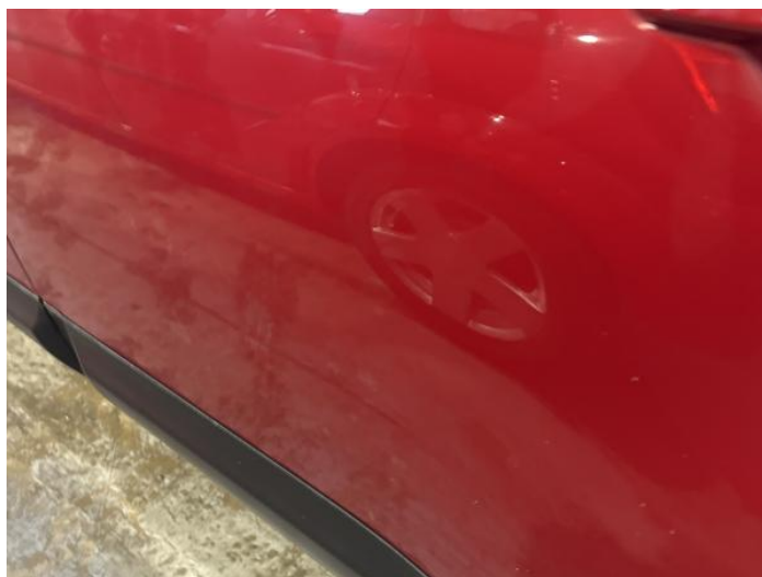
6: Door nsr Dented With Paint Damage
