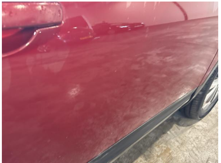
12: Door osf Dented Over 2 UpTo 10mm
