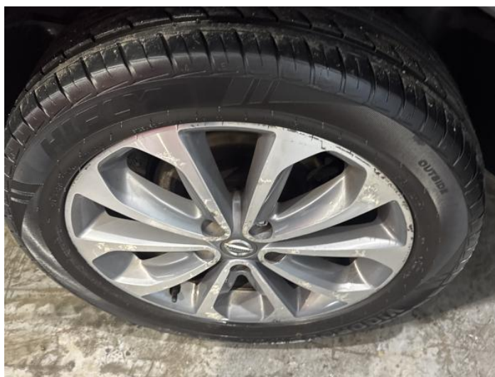
8: Wheel nsf Scratched Over 50mm
