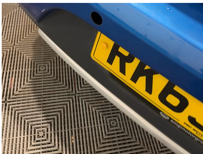
12: Parking Sensor Rear Missing Replace
