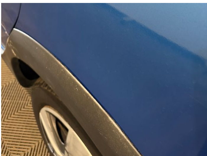
11: Qtr Panel nsr Poor Previous Repair Rippled UpTo 30%
