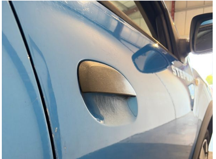
16: Door osf Dented With Paint Damage
