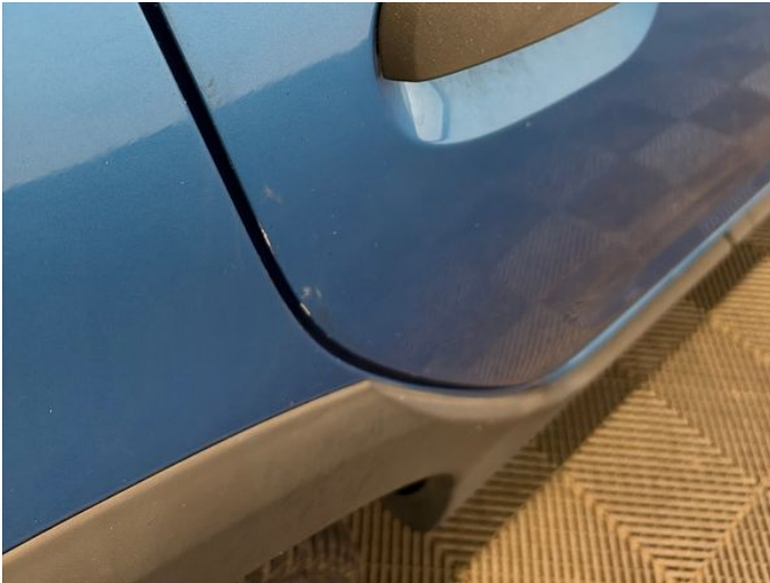
15: Door osr Dented With Paint Damage
