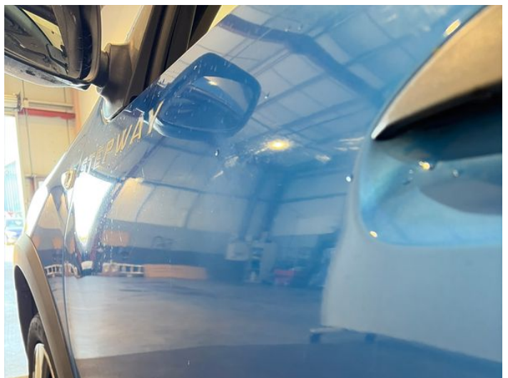
8: Door nsf Dented Over 30mm
