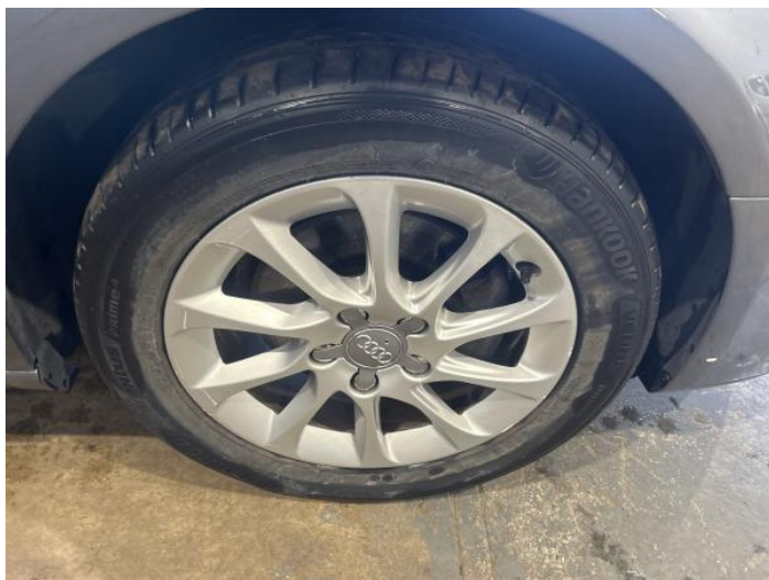
1: Wheel osf Scratched Over 50mm
