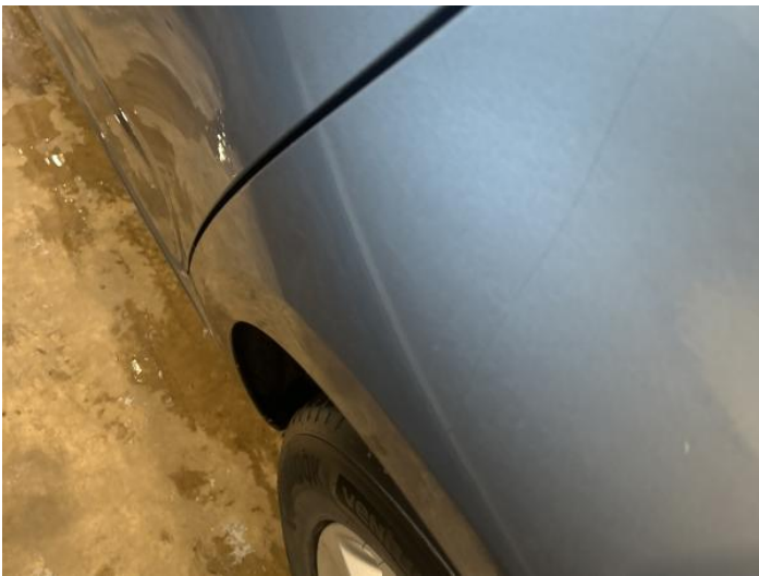
5: Qtr Panel nsr Dented Between 10mm + 30mm
