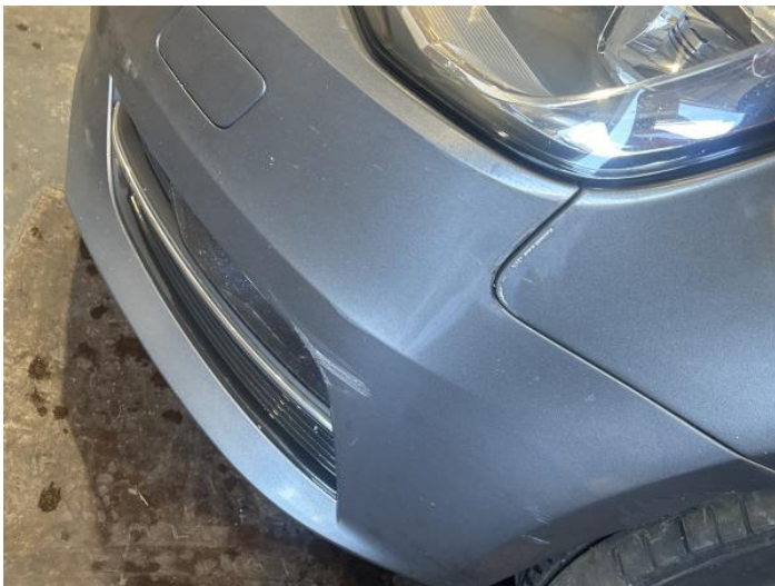
10: Bumper Front Scratched Over 100mm Thru Paint
