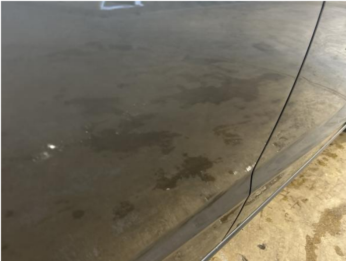
3: Door osr Dented Over 30mm
