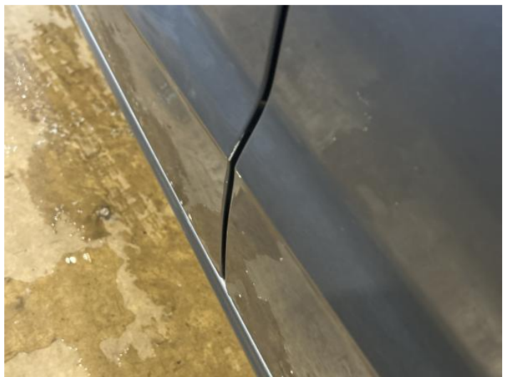
8: Door nsf Chipped Edge Chip
