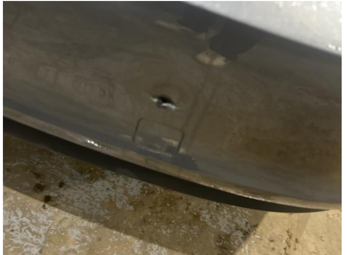
4: Bumper Rear Hole UpTo 25mm
