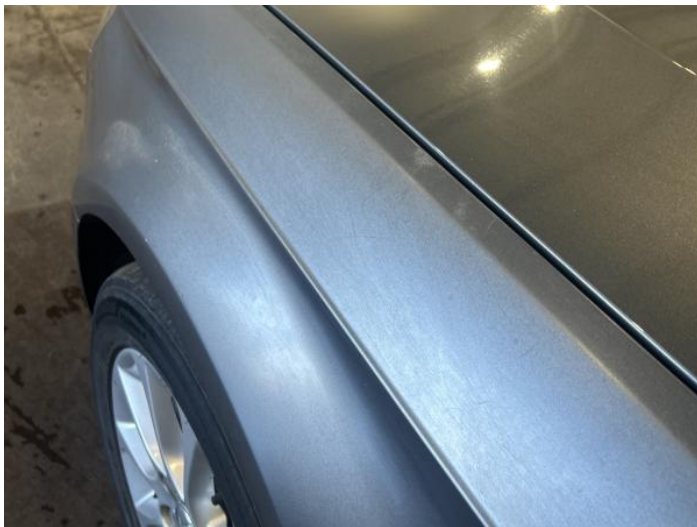
9: Wing nsf Poor Previous Repair Poor Paint
