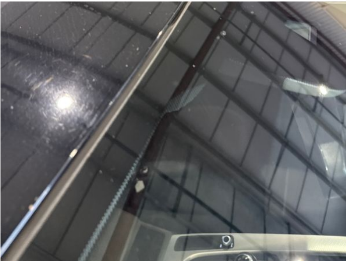
18: Roof Chipped Edge Chip
