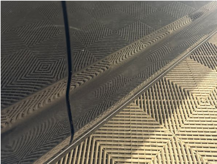
15: Door osf Scratched UpTo 25mm Thru Paint
