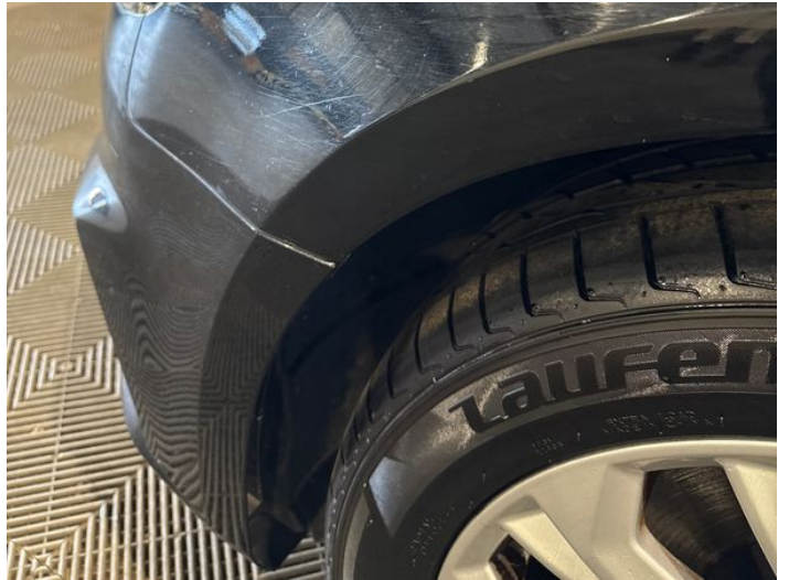
4: Wing nsf Chipped Multiple Chips
