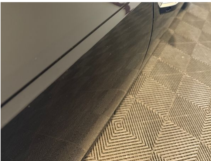
13: Door osr Dented Between 10mm + 30mm
