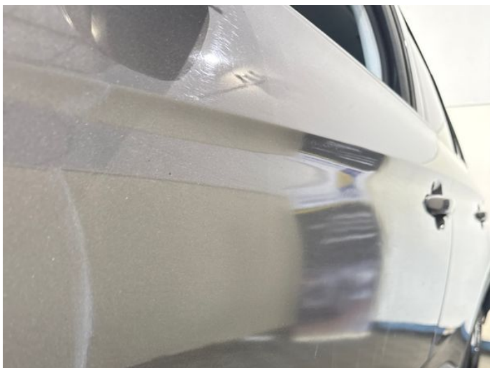
3: Door nsf Poor Previous Repair Rippled Up To 30%
