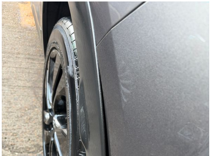
16: Qtr Panel Arch Extension ns Broken Replace
