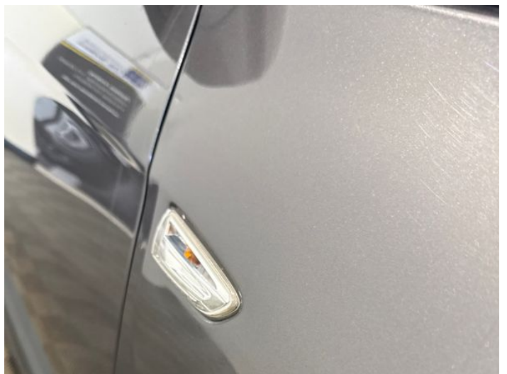
14: Wing osf Dented Over 30mm
