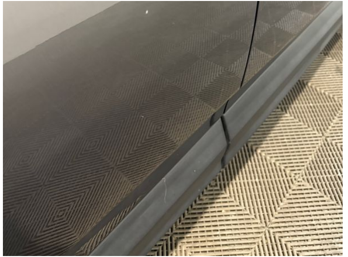
10: Door osr Dented Between 10mm + 30mm
