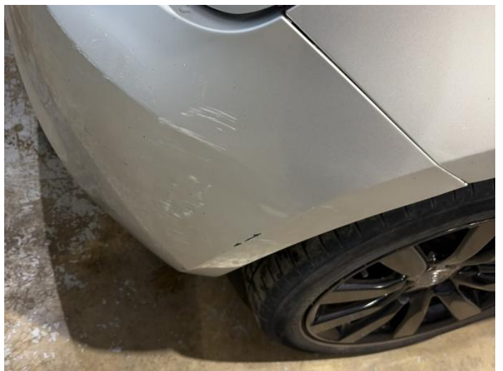
8: Bumper Rear Poor Previous Repair Paint Flake
