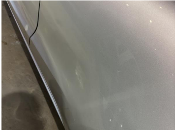
10: Qtr Panel nsr Poor Previous Repair Poor Paint
