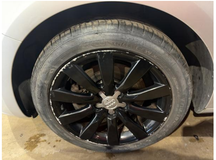
12: Wheel nsf Scratched Over 50mm
