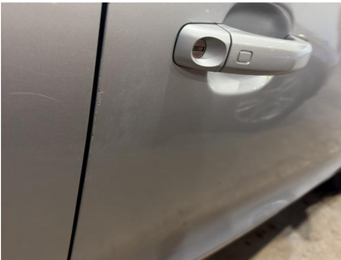
5: Door osf Chipped Edge Chip
