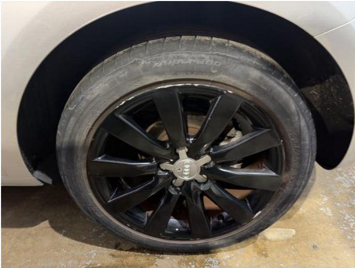
9: Wheel nsr Scratched Over 50mm
