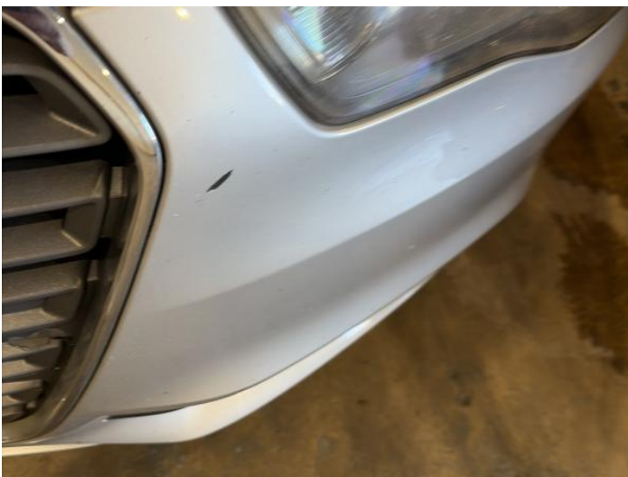
13: Bumper Front Scratched UpTo 25mm Thru Paint
