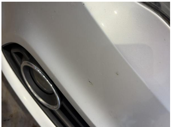
14: Bumper Front Chipped Multiple Chips
