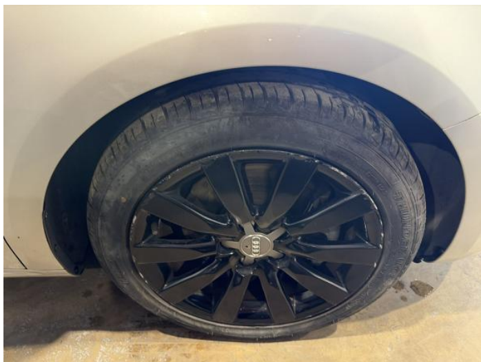
1: Wheel of Scratched Over 50mm
