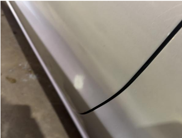
11: Door nsf Poor Previous Repair Poor Paint
