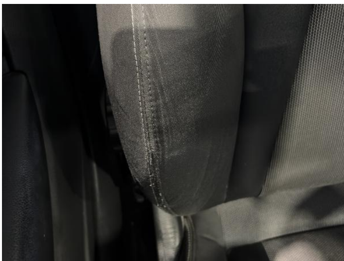
17: Seat Back Cover osf Scuffed Over 25mm
