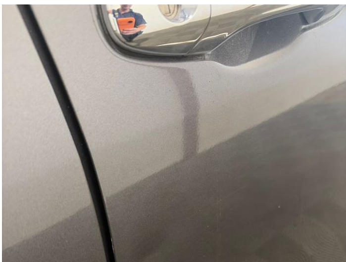
13: Door osf Dented Between 10mm + 30mm
