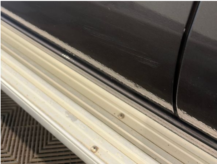
5: Door nsf Scratched Over 25mm Thru Paint
