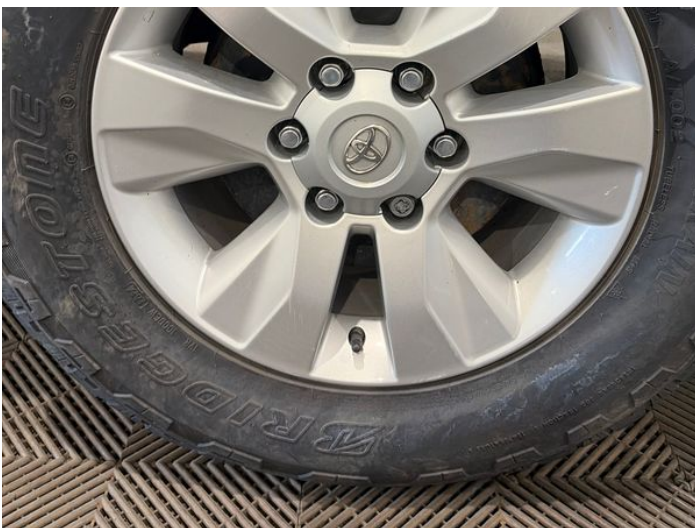
7: Wheel nsr Scratched Over 50mm
