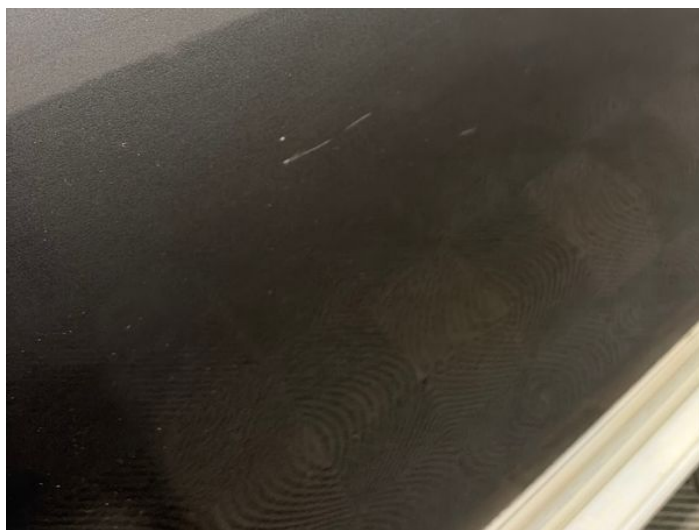
12: Door osr Scratched Over 25mm Thru Paint
