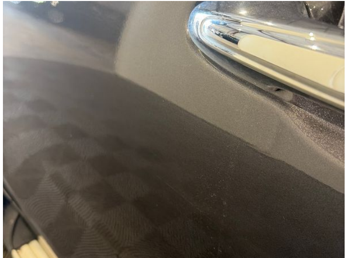
4: Door nsf Dented Over 30mm
