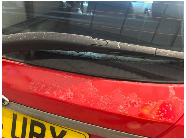
4: Tailgate Poor Previous Repair Paint Flake
