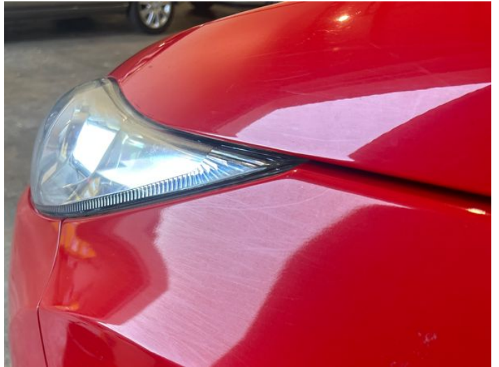
10: Wing nsf Poor Previous Repair Poor Paint
