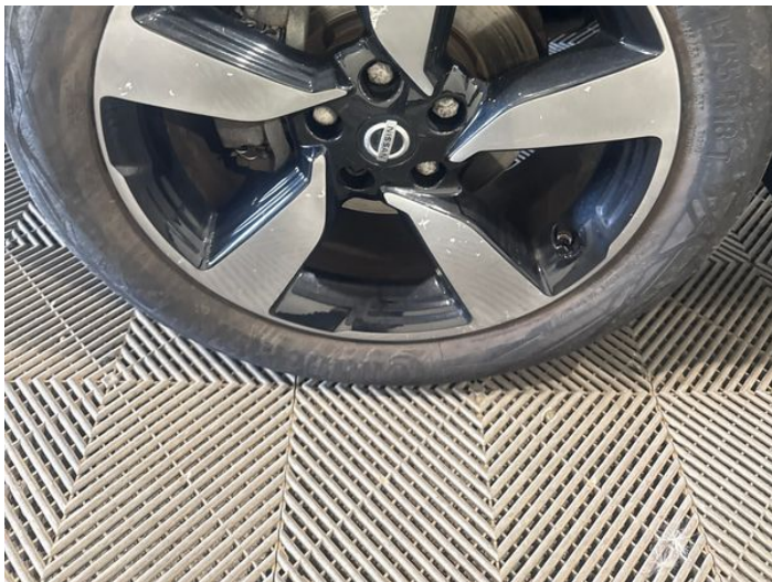
3: Wheel nsf Corroded Light
