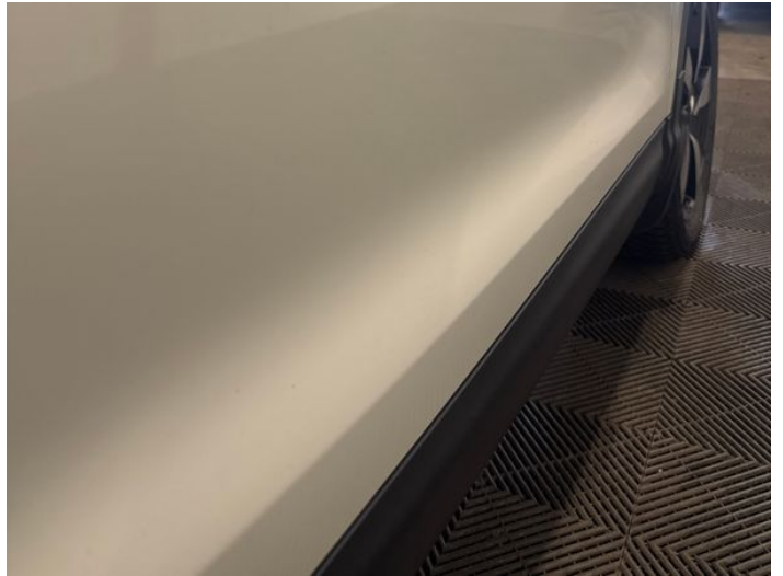
10: Door osf Dented Over 30mm
