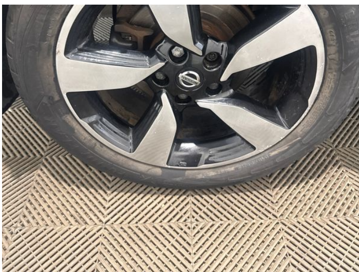
7: Wheel osr Scratched Over 50mm
