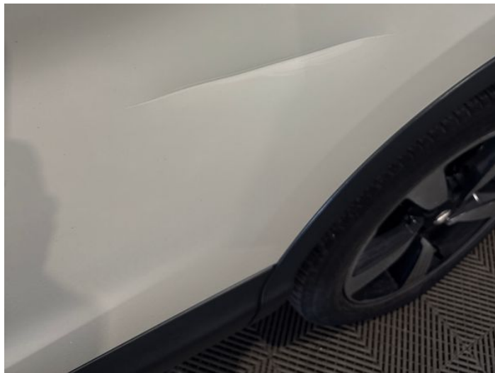
4: Door nsr Dented With Paint Damage
