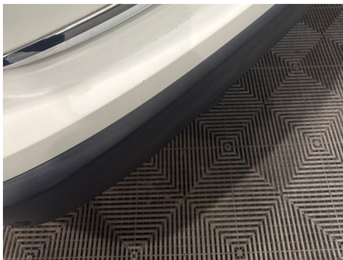
6: Bumper Rear Scratched 25 to 100mm Thru Paint
