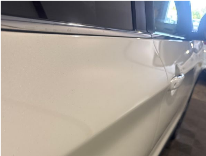
9: Door osr Dented Between 10mm + 30mm
