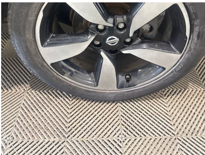
5: Wheel nsr Corroded Light
