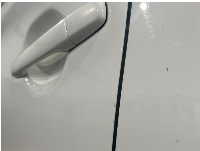
9: Door nsr Chipped Edge Chip
