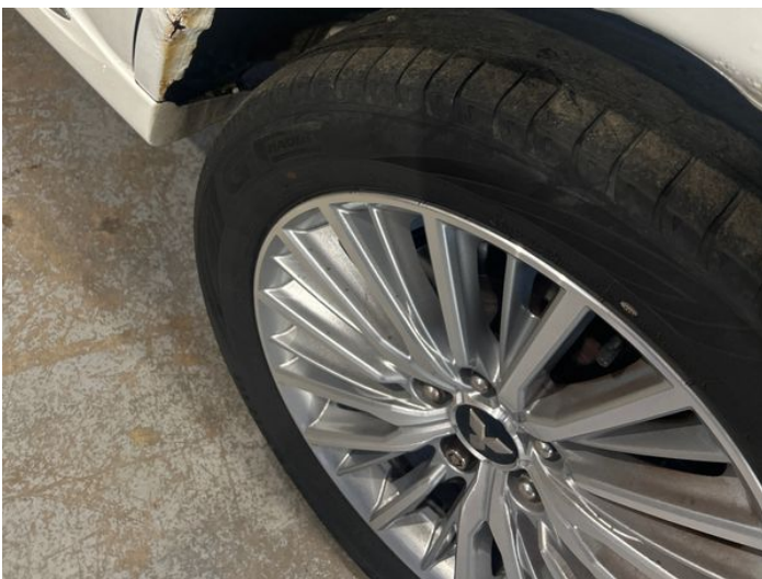
7: Qtr Panel nsr Rusted Over 5mm
