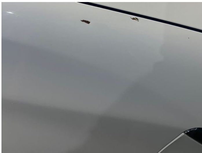
1: Wing osf Chipped Over 5mm
