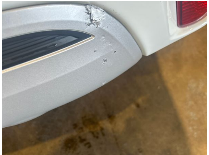
6: Bumper Rear Moulding Broken Replace
