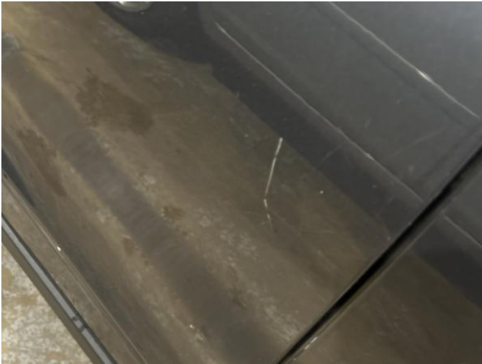
3: Door osr Scratched Over 25mm Thru Paint
