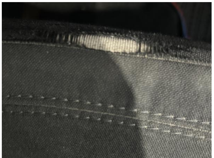
14: Seat Base Cover osf Torn UpTo 3mm
