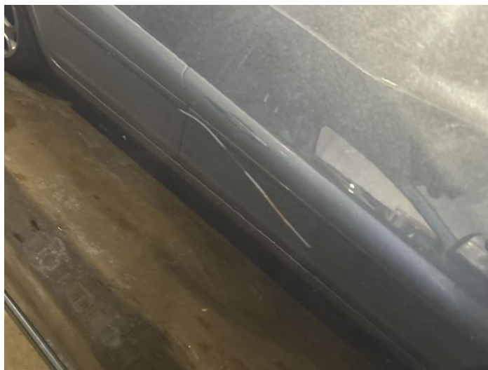
2: Door osf Scratched Over 25mm Thru Paint
