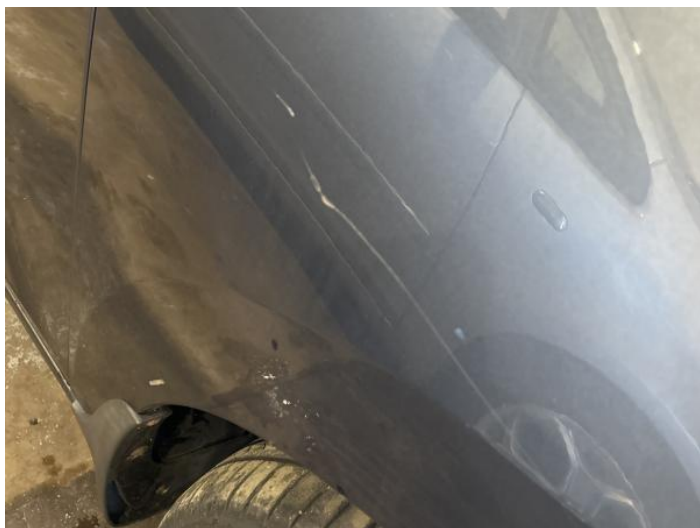
1: Wing osf Scratched Over 25mm Thru Paint
