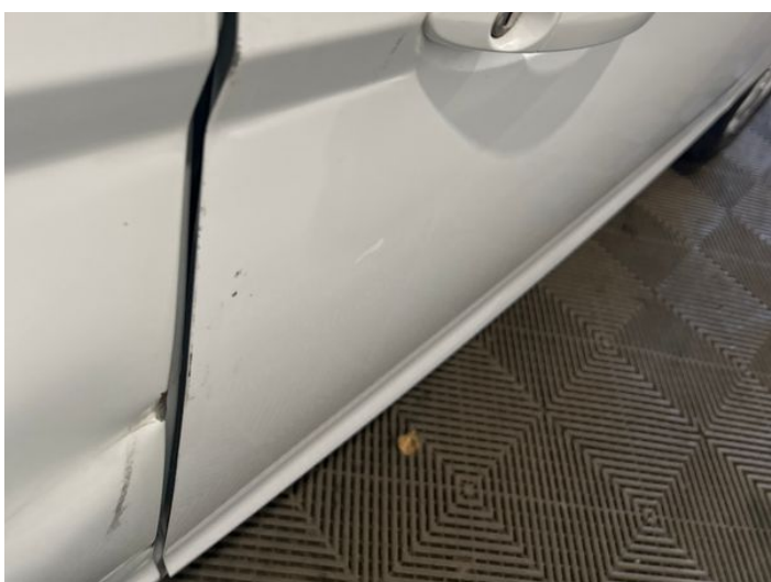
13: Door osf Chipped Edge Chip
