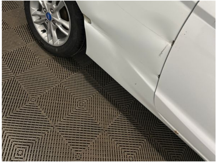
4: Qtr Panel osr Dented Over 30% Of Panel
