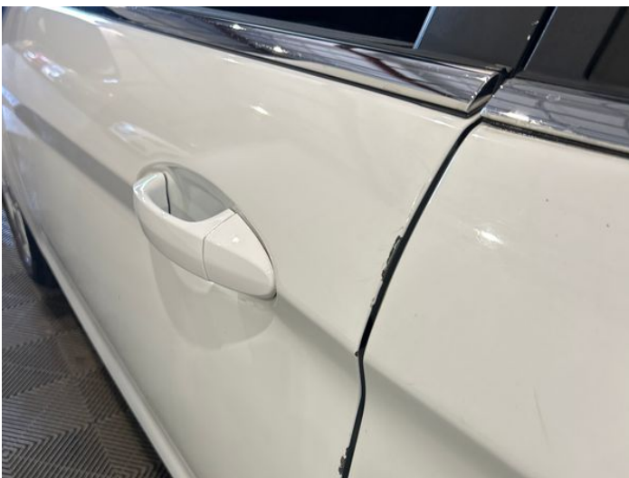
7: Door nsf Chipped Edge Chip
