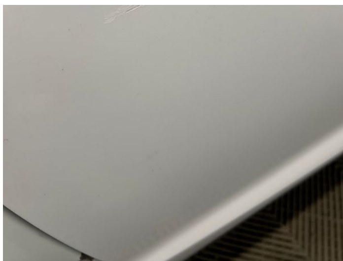
12: Door osf Scratched UpTo 25mm Thru Paint
