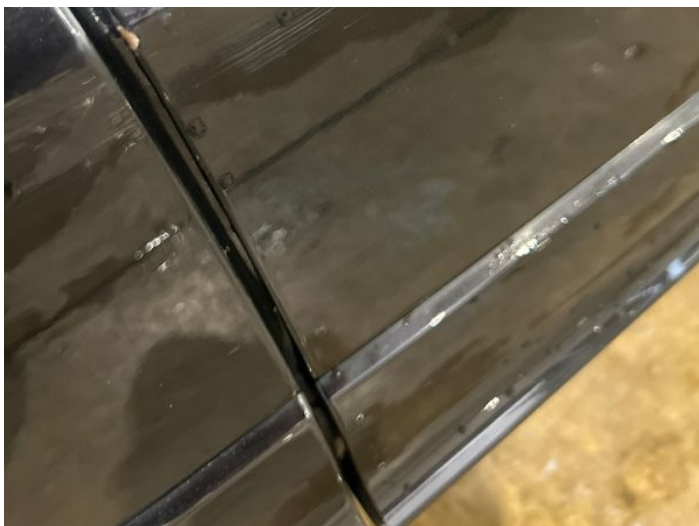
3: Door osf Scratched UpTo 25mm Thru Paint
