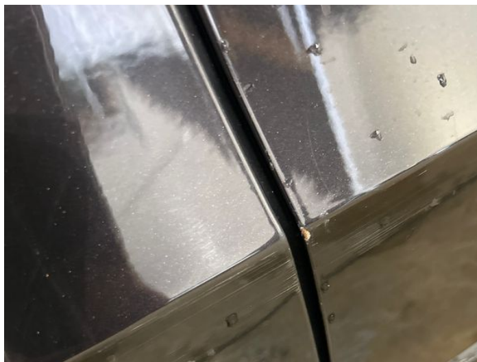
2: Door osr Scratched UpTo 25mm Thru Paint
