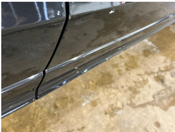
1: Door osf Chipped Edge Chip
