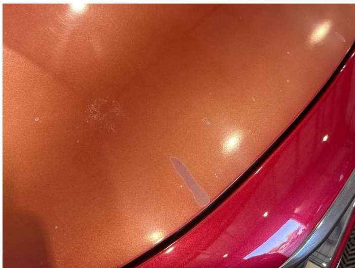
1: Bonnet Poor Previous Repair Paint Flake
