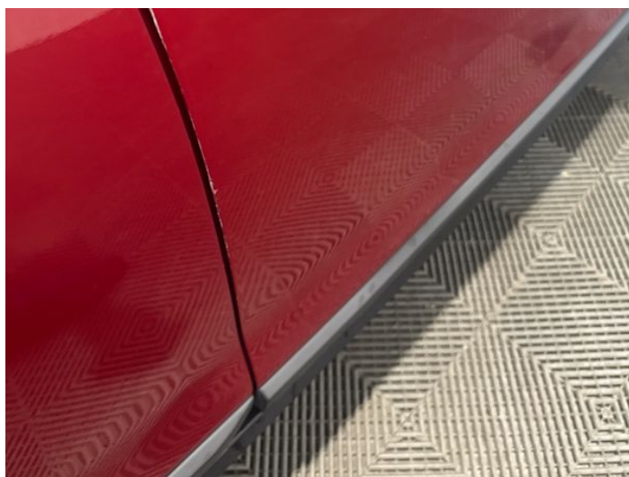
14: Door osf Chipped Edge Chip
