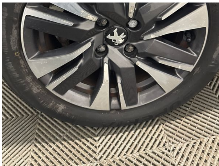
12: Wheel osr Corroded Light
