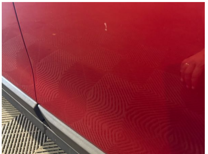
8: Door nsr Scratched Over 25mm Thru Paint
