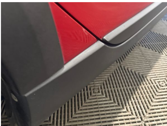
13: Door osr Scratched UpTo 25mm Thru Paint
