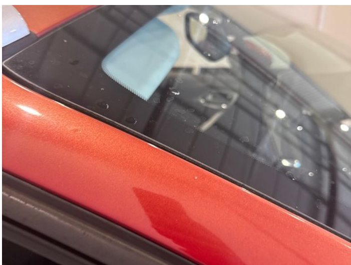
17: A Post os Chipped 1 To 5
