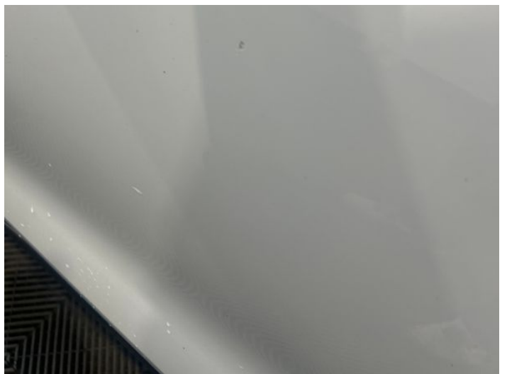
8: Door nsf Chipped 1 To 5
