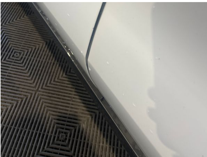
7: Door nsf Chipped Edge Chip
