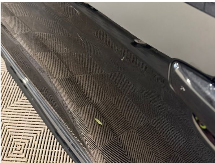
7: Door nsr Scratched Over 25mm Thru Paint
