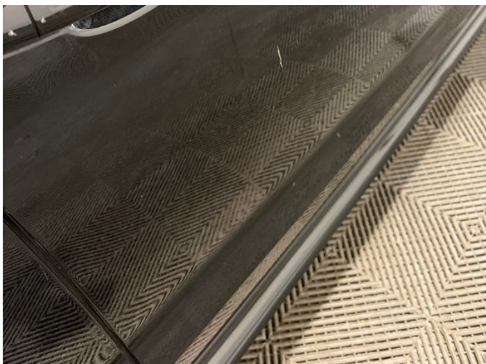
15: Door osf Scratched Over 25mm Thru Paint
