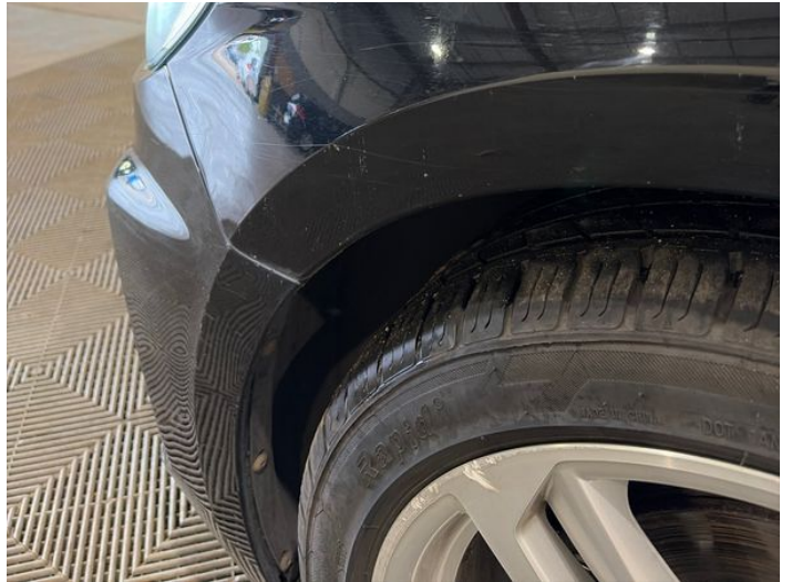
4: Wing nsf Scratched Over 25mm Thru Paint
