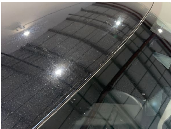
16: Roof Chipped Edge Chip
