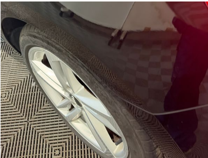
11: Qtr Panel nsr Dented Between 10mm + 30mm
