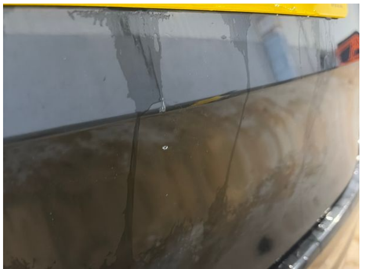
8: Tailgate Poor Previous Repair Poor Paint
