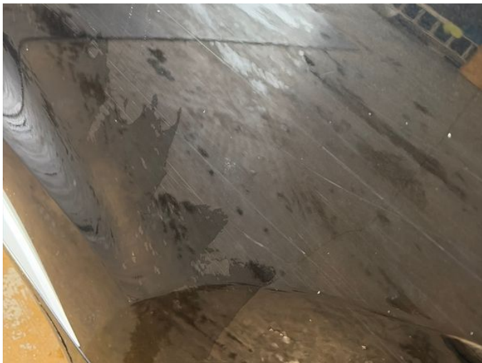
9: Door nsr Scratched Over 25mm Thru Paint
