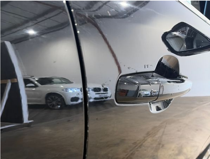
3: Door osf Chipped Edge Chip
