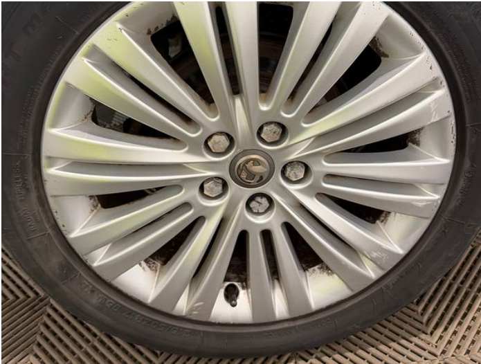
15: Wheel osr Scratched Over 50mm
