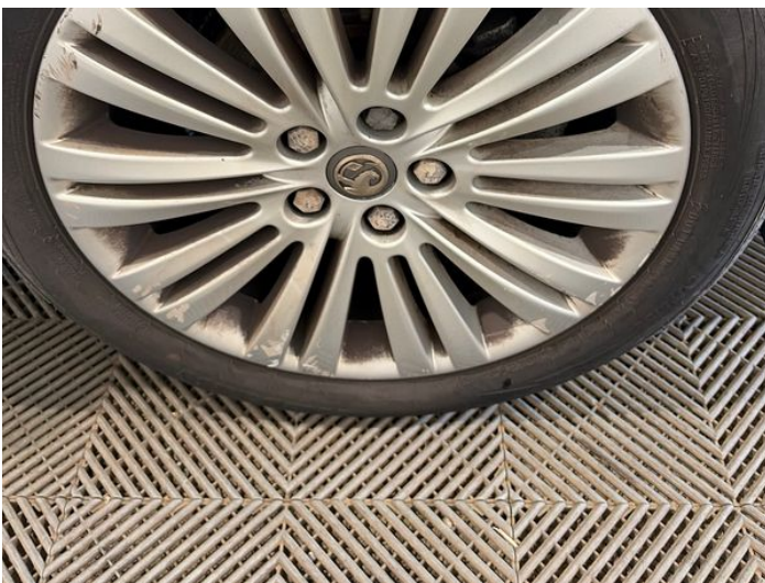
19: Wheel osf Scratched Over 50mm
