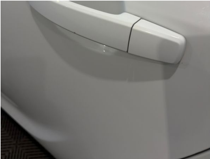
9: Handle Outer nsr Scratched (Painted) UpTo 25mm Thru Paint
