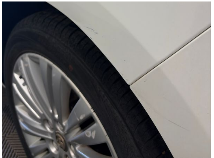
12: Qtr Panel nsr Scratched UpTo 25mm Thru Paint
