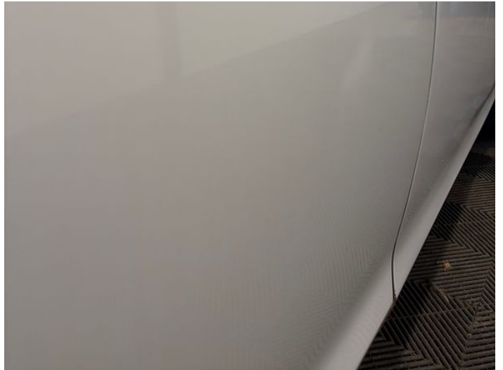
16: Door osr Dented Between 10mm + 30mm
