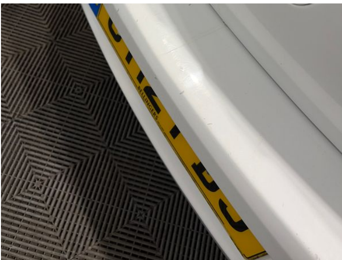
13: Bumper Rear Scratched Over 100mm Thru Paint
