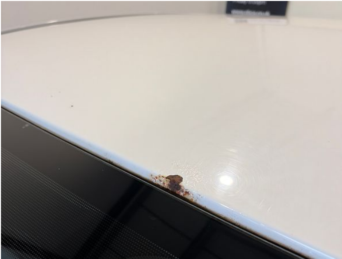
3: Roof Rusted Over 5mm
