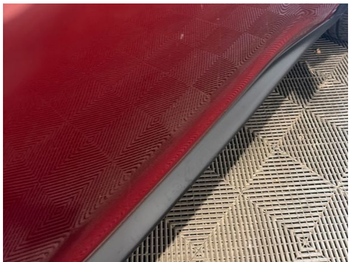
14: Door osf Scratched Over 25mm Thru Paint
