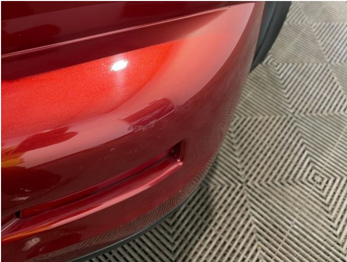
9: Bumper Rear Scratched 25 to 100mm Thru Paint
