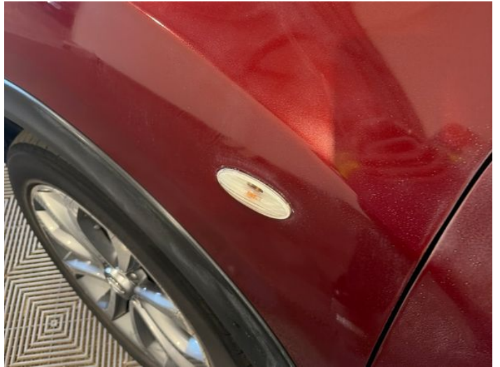
4: Wing nsf Poor Previous Repair Poor Paint
