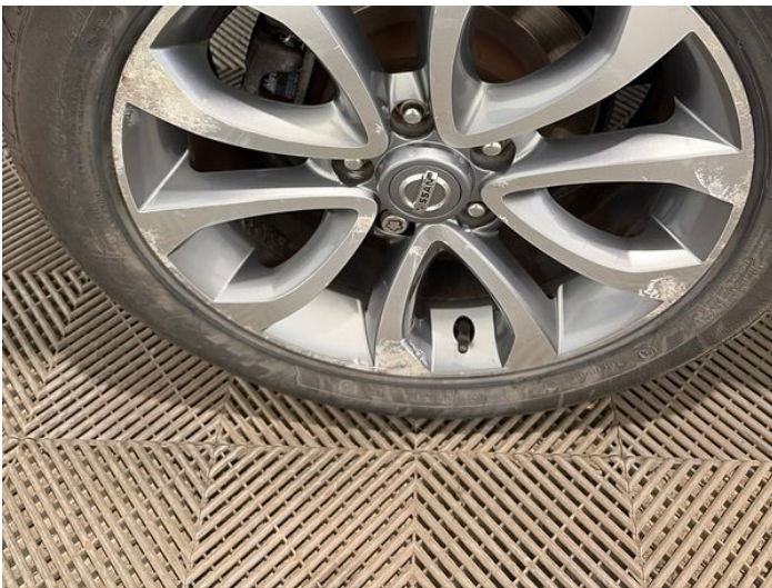
11: Wheel osr Scratched Over 50mm
