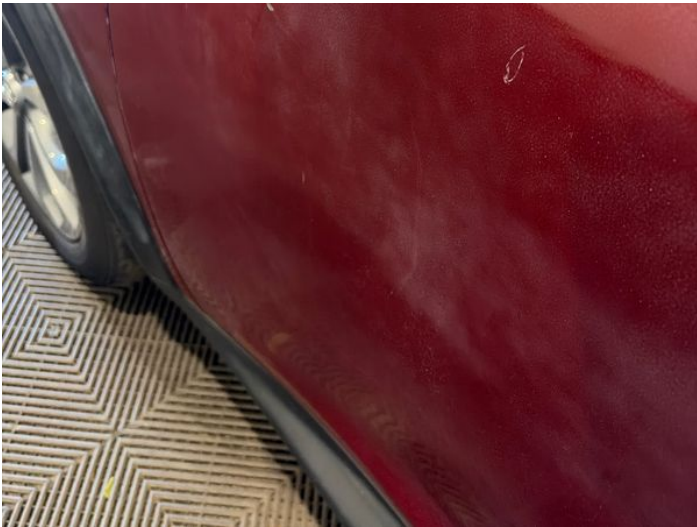
5: Door nsf Poor Previous Repair Rippled UpTo 30%
