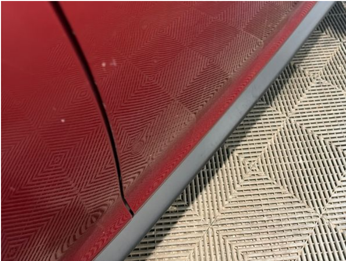
15: Door osf Dented Between 10mm + 30mm
