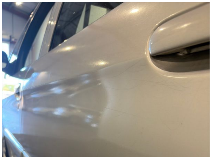
8: Door nsr Poor Previous Repair Rippled UpTo 30%
