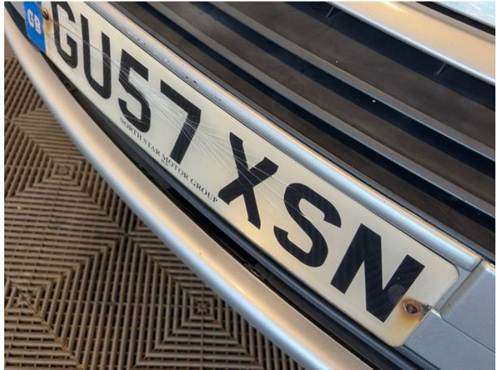
4: Number Plate Front Broken Replace
