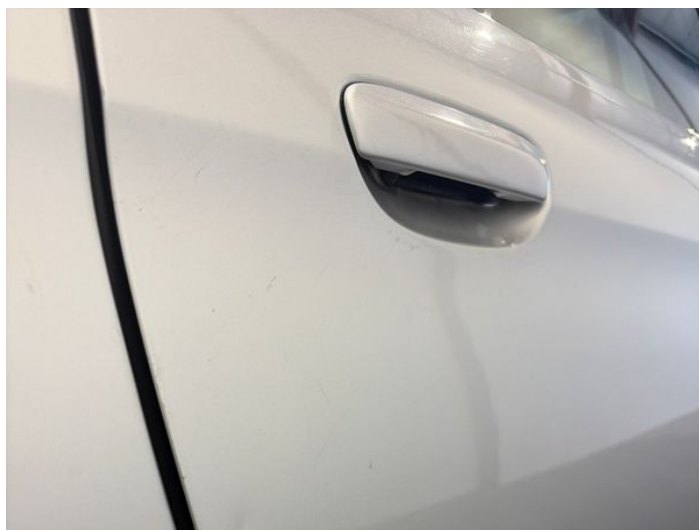
18: Door osr Dented Between 10mm + 30mm
