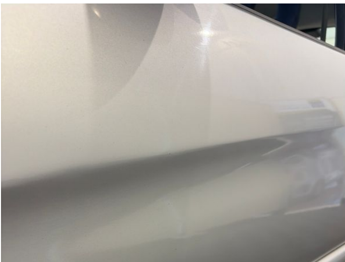
7: Door nsf Poor Previous Repair Poor Paint
