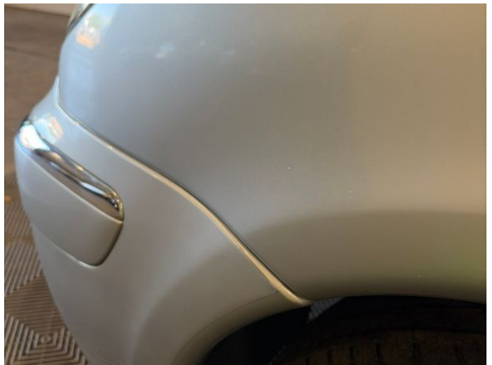
6: Wing nsf Poor Previous Repair Poor Paint
