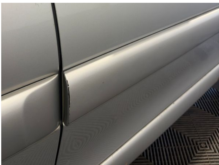
19: Door osf Scratched Over 25mm Thru Paint
