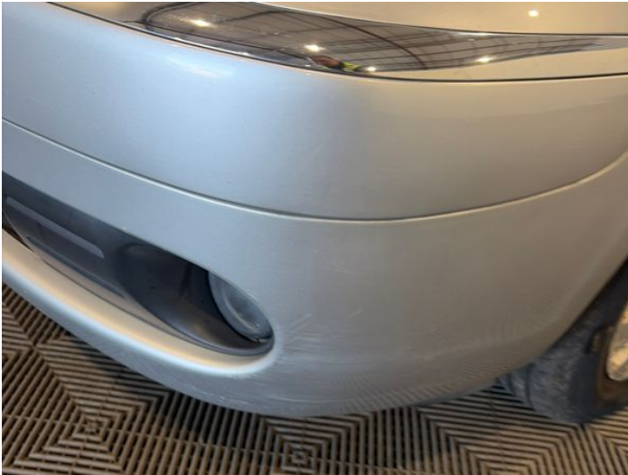
3: Bumper Front Scratched Over 100mm Thru Paint
