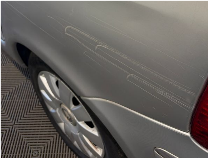
9: Qtr Panel nsr Dented With Paint Damage
