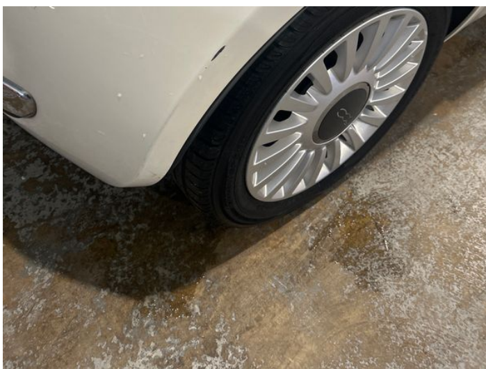
7: Bumper Rear Scratched Up To 25mm Thru Paint
