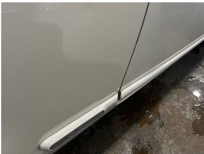
5: Qtr Panel osr Dented Between 10mm + 30mm
