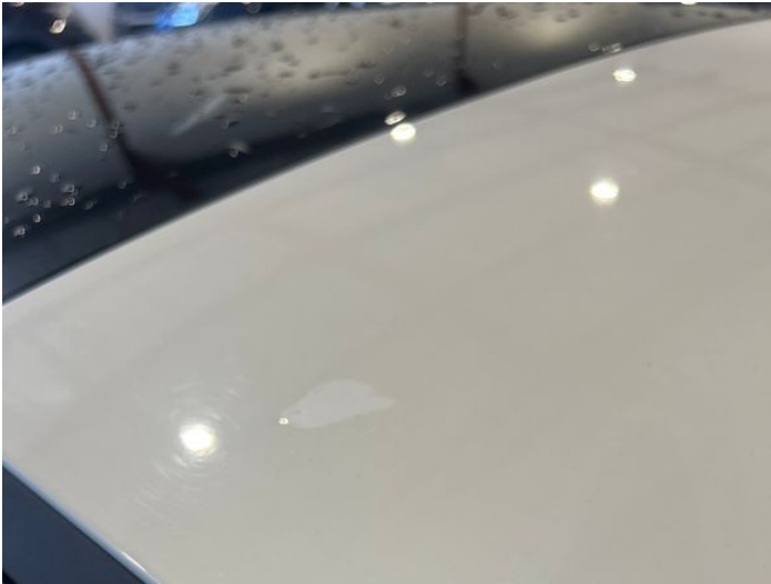
9: Roof Poor Previous Repair Paint Flake
