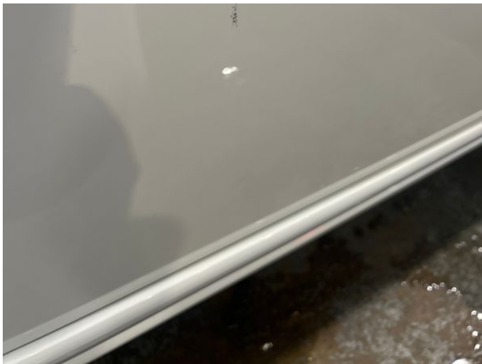
3: Door osf Scratched Up To 25mm Thru Paint
