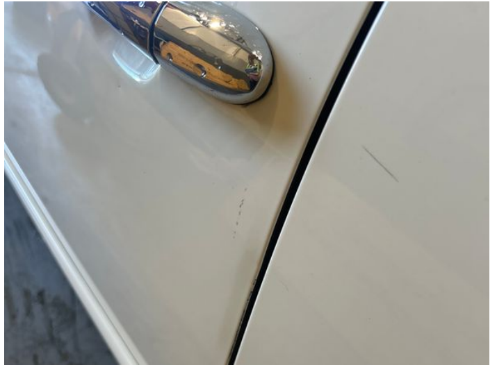
10: Door nsf Dented Over 30mm
