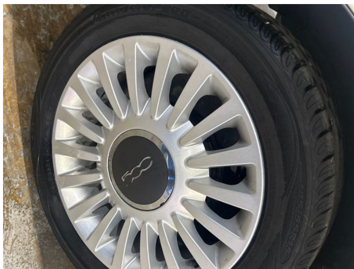
6: Wheel osr Scratched Up To 50mm
