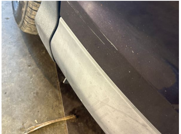
12: Bumper Front Scratched 25 to 100mm Thru Paint
