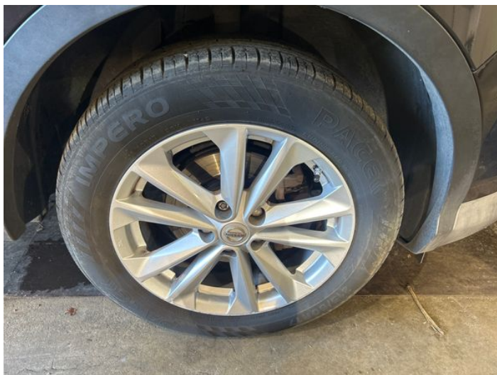
1: Wheel osf Scratched Over 50mm
