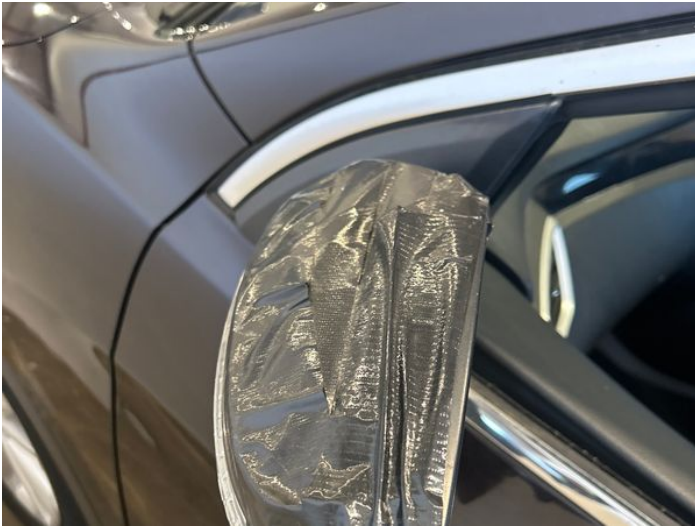
9: Door Mirror Assy nsf Broken Replace
