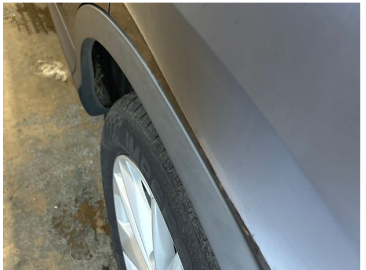
6: Qtr Panel nsr Dented Between 10mm + 30mm
