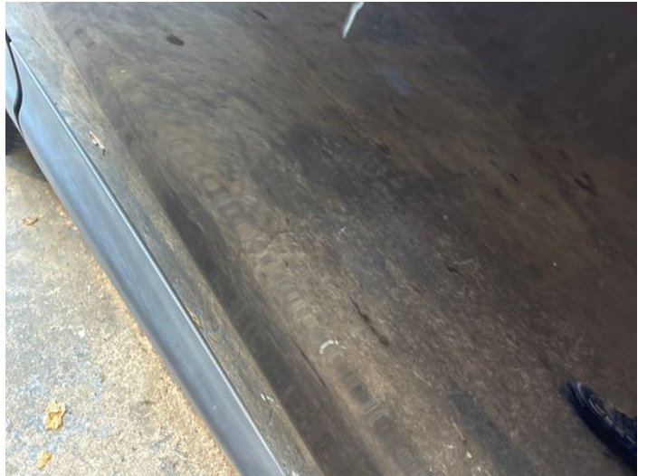
4: Door osr Scratched Over 25mm Thru Paint
