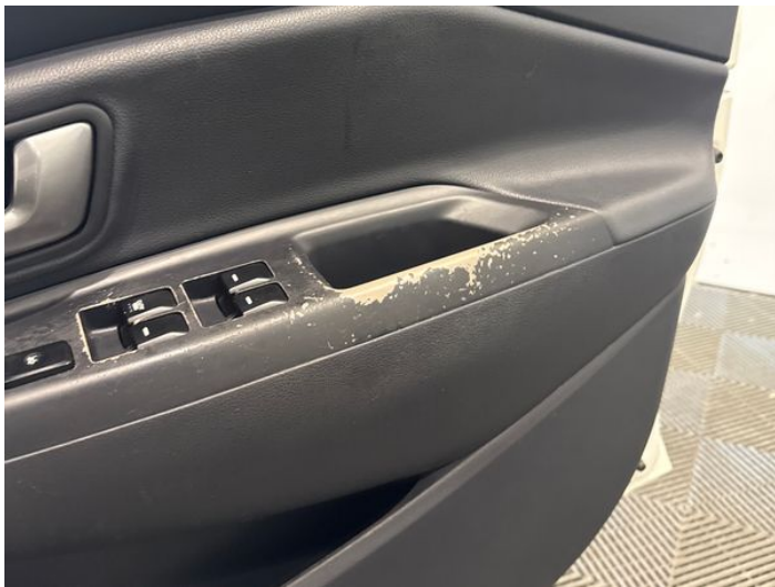
17: Door Pad osf Scuffed Over 25mm
