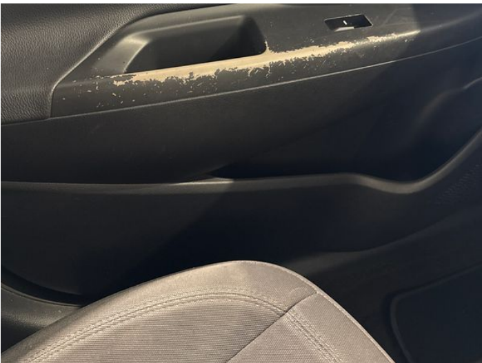
16: Door Pad nsf Scuffed Over 25mm
