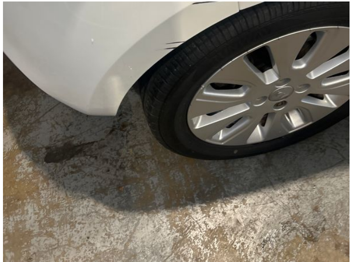
6: Bumper Rear Scratched 25 to 100mm Thru Paint
