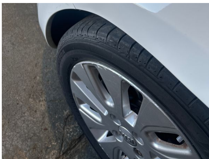
12: Wing nsf Dented Over 30mm
