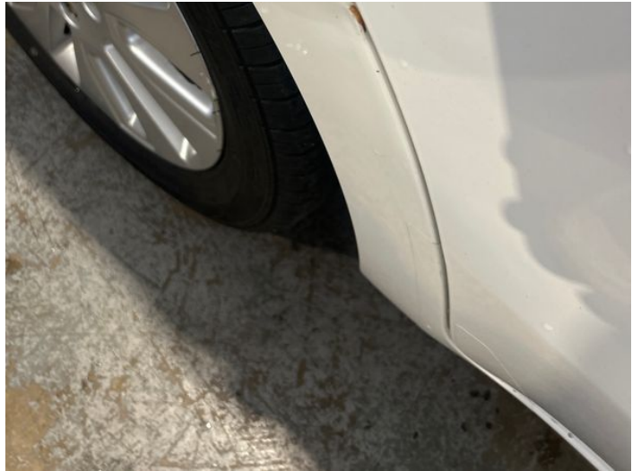
4: Qtr Panel osr Dented With Paint Damage
