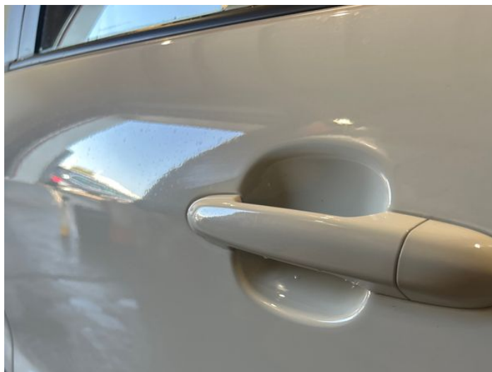
10: Door nsr Poor Previous Repair Poor Paint
