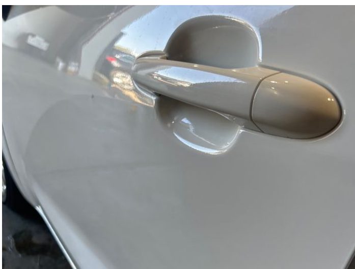
11: Door nsf Poor Previous Repair Poor Paint
