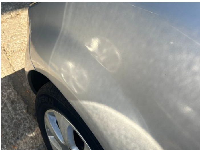
9: Wing nsf Poor Previous Repair Poor Paint
