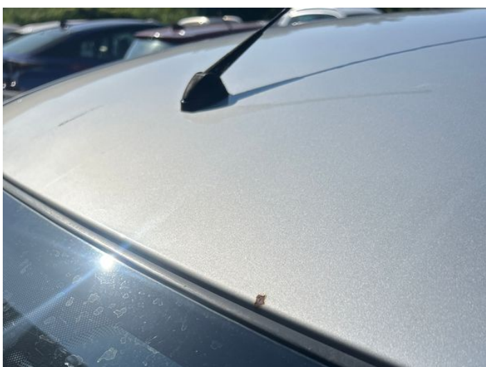
13: Roof Chipped 1 To 5
