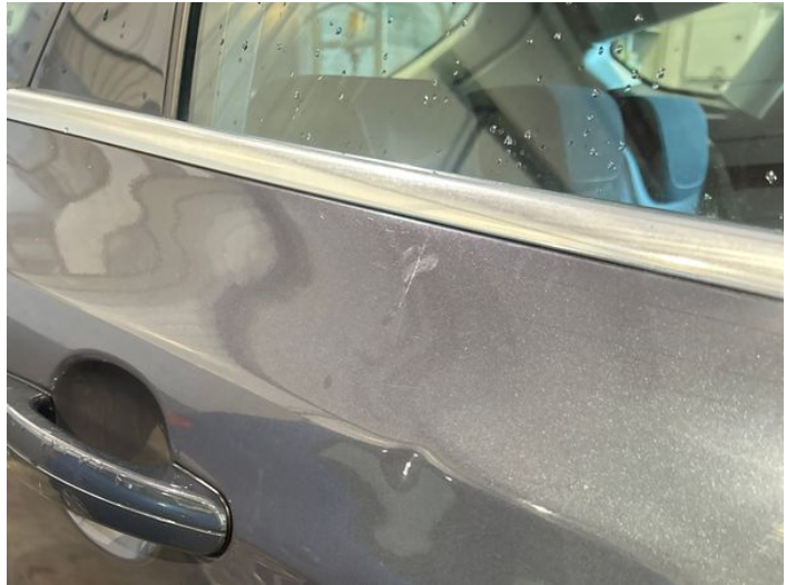
4: Door osr Dented Over 30mm
