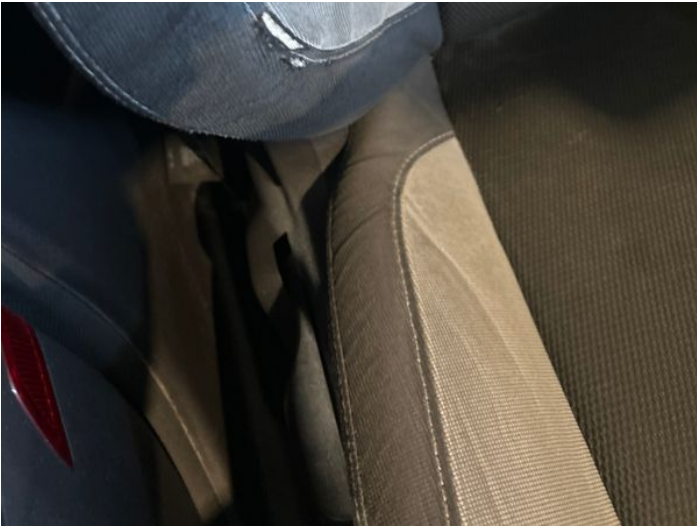
16: Seat Back Cover osf Torn UpTo 3mm
