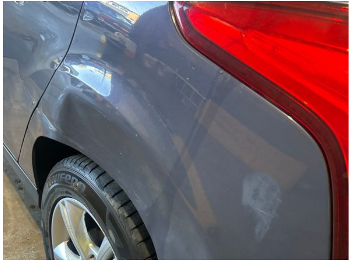
10: Qtr Panel nsr Dented Over 30% Of Panel
