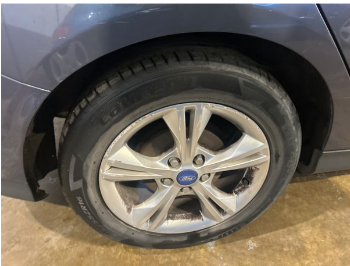
7: Wheel osr Scratched Over 50mm
