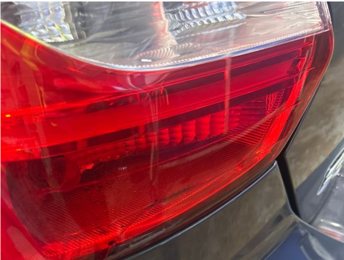
18: Lamp nsr Broken Replace
