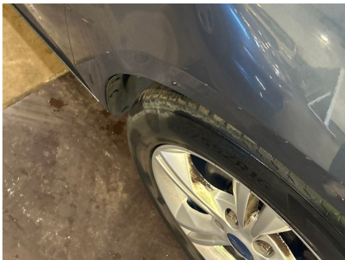
1: Wing osf Dented Over 30mm
