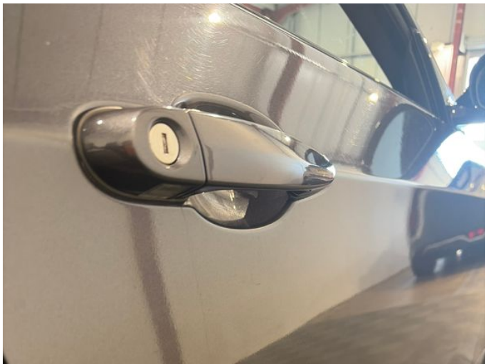
11: Door osf Poor Previous Repair Poor Paint
