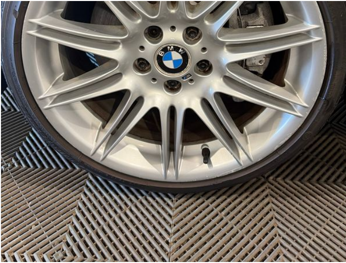
3: Wheel nsf Scratched Over 50mm
