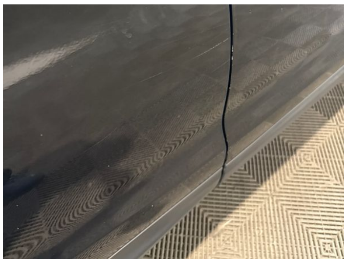
14: Door osr Scratched Over 25mm Thru Paint
