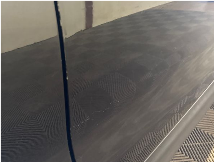
15: Door osf Dented Between 10mm + 30mm
