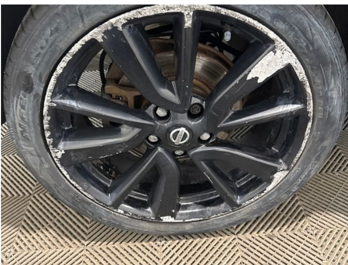
13: Wheel osr Scratched Over 50mm
