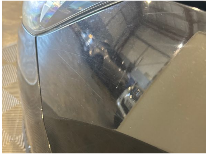
4: Wing nsf Scratched UpTo 25mm Thru Paint
