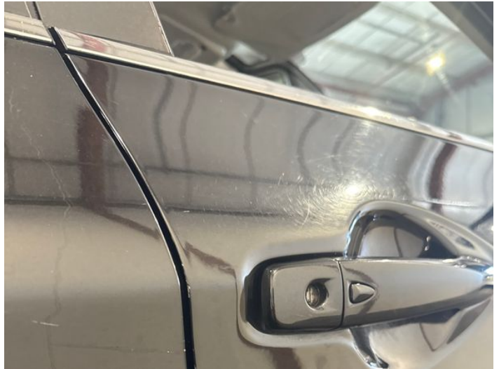
16: Door osf Chipped Edge Chip
