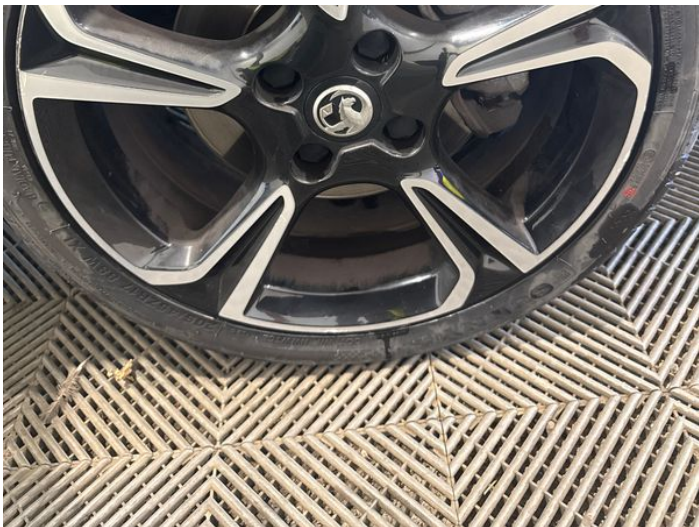
18: Wheel osf Scratched Over 50mm
