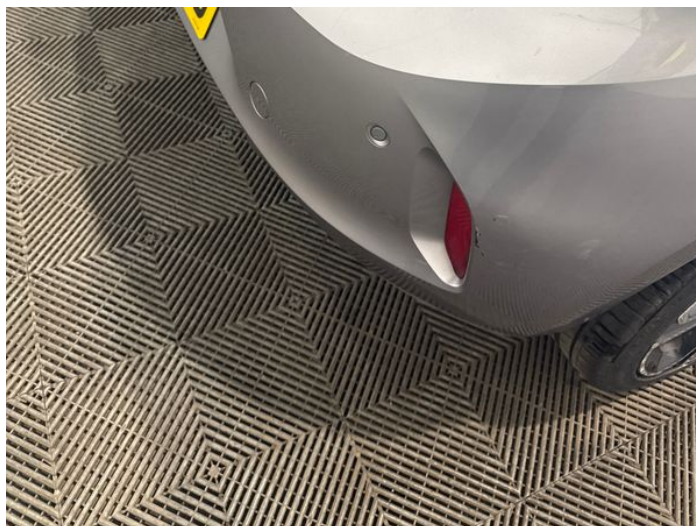
10: Bumper Rear Scratched Over 100mm Thru Paint
