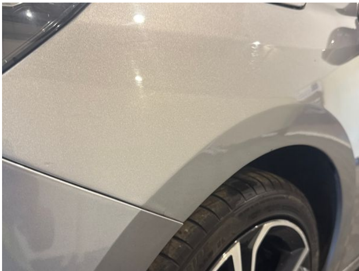
3: Wing nsf Poor Previous Repair Rippled UpTo 30%
