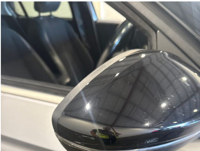
16: Door Mirror Assy osf Scratched (Painted) Over 25mm Thru Paint
