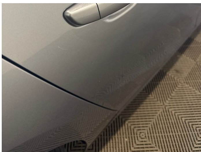
14: Door osr Scratched Over 25mm Thru Paint
