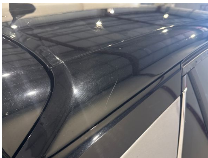
12: C Post os Scratched Over 25mm Thru Paint
