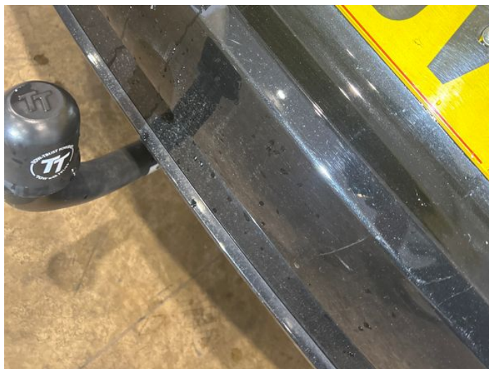
4: Bumper Rear Moulding Scratched (Painted) Over 25mm Thru Paint
