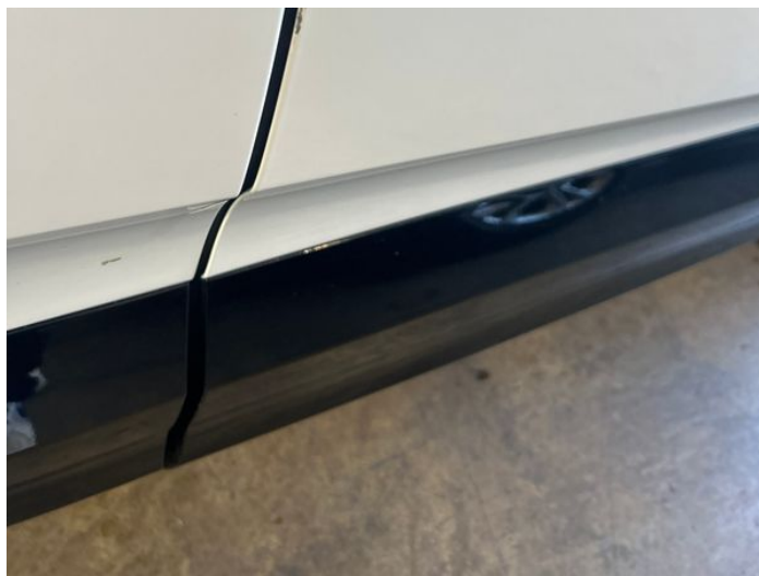
2: Door osf Chipped Edge Chip
