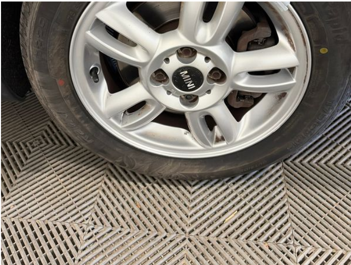
11: Wheel osf Scratched Over 50mm
