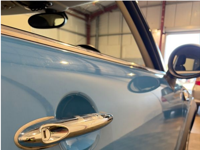
10: Door osf Dented Over 30mm
