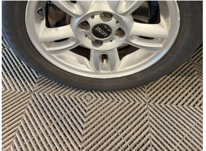
4: Wheel nsf Scratched Over 50mm
