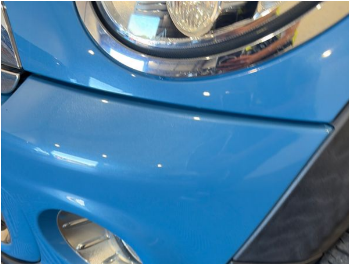
3: Bumper Front Scratched UpTo 25mm Thru Paint
