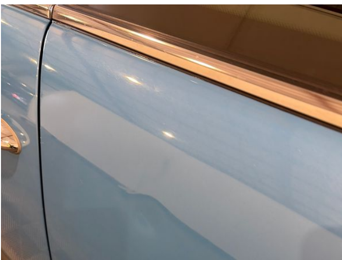
7: Qtr Panel nsr Dented Over 30mm
