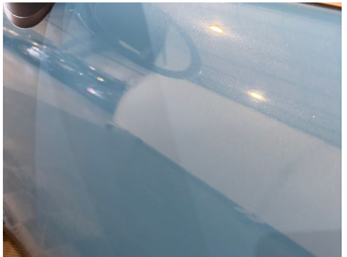
6: Door nsf Dented Over 30mm
