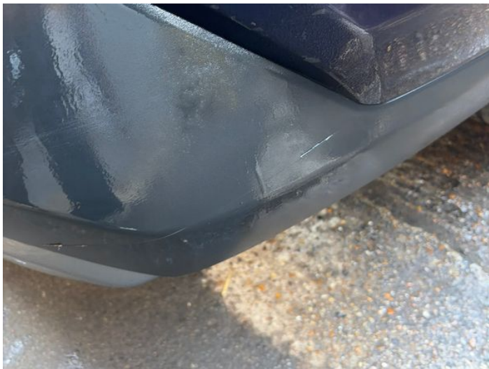
15: Bumper Rear Moulding Scuffed (Unpainted) UpTo 100mm
