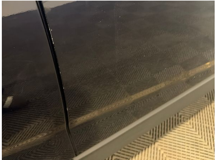
10: Door osf Chipped Edge Chip
