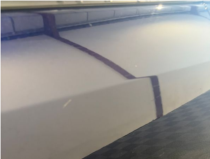
9: Door osr Scratched Over 25mm Thru Paint
