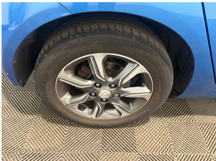
3: Wheel osr Corroded Light
