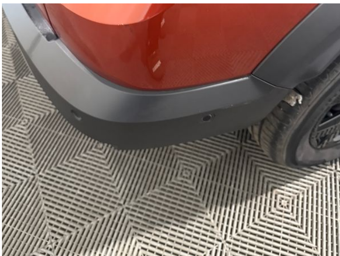
15: Bumper Rear Scratched 25 to 100mm Thru Paint
