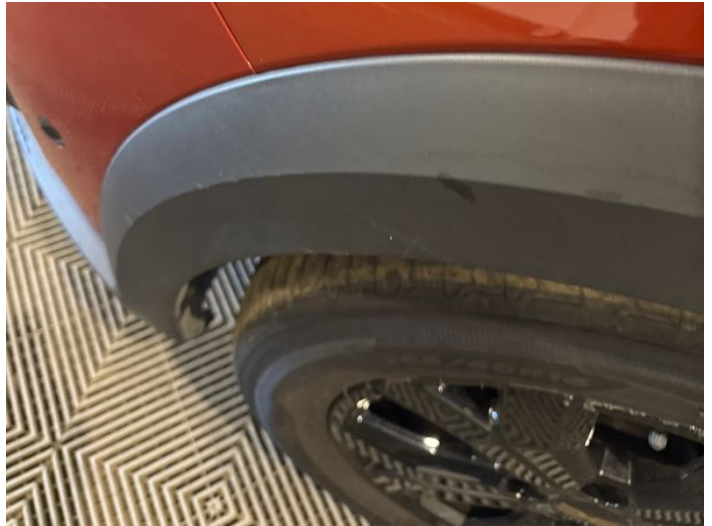
4: Wing nsf Scratched Over 25mm Thru Paint
