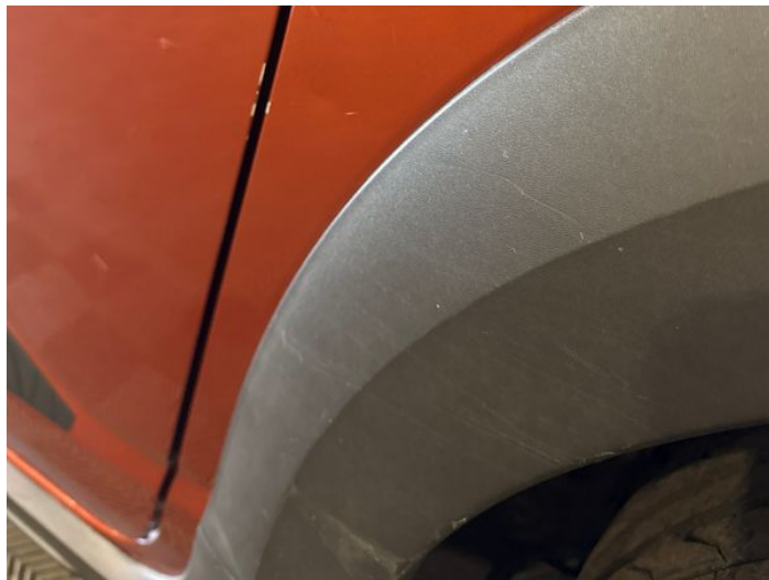
10: Qtr Panel nsr Dented Between 10mm + 30mm
