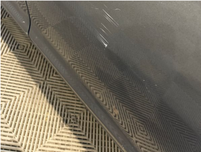
9: Door nsr Scratched Over 25mm Thru Paint
