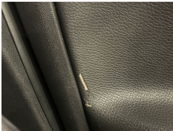
2: Door Pad nsf Torn Between 3mm + 10mm
