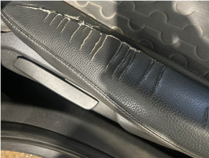
3: Seat Base Cover osf Torn Over 3mm
