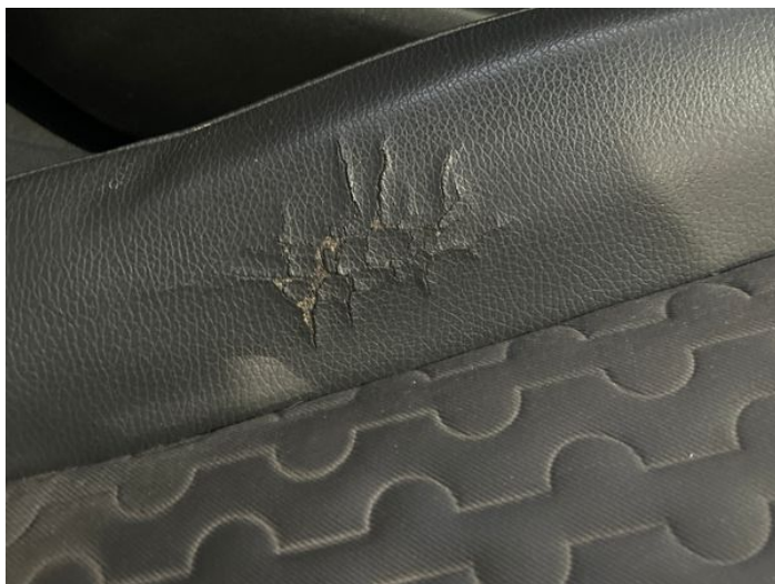
1: Seat Base Cover nsf Torn Over 3mm
