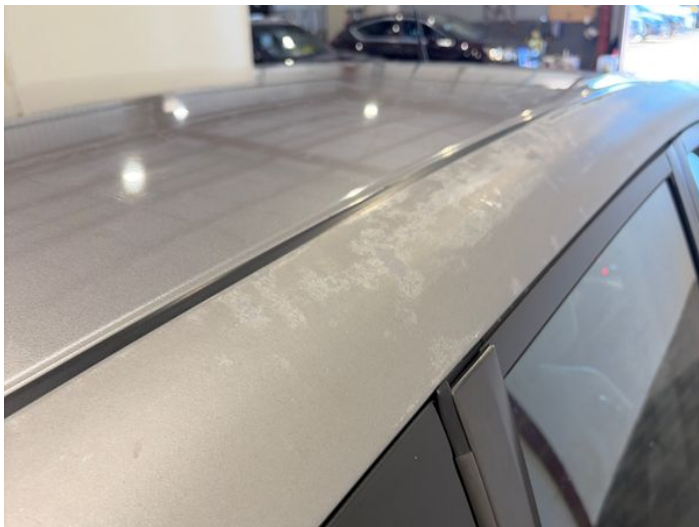
15: B Post os Poor Previous Repair Paint Flake
