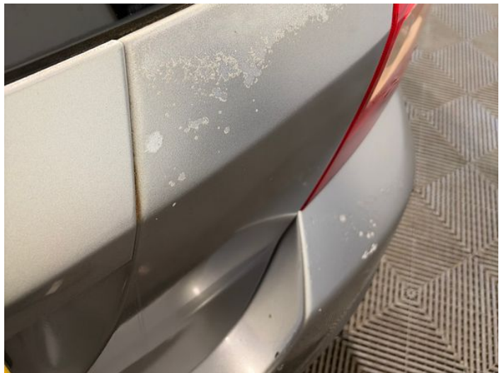
12: Tailgate Poor Previous Repair Poor Paint
