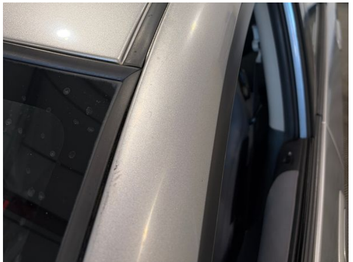
6: A Post ns Poor Previous Repair Poor Paint
