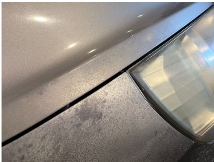
1: Bonnet Poor Previous Repair Poor Paint
