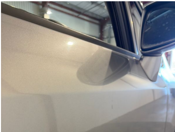
17: Door osf Dented Over 30mm
