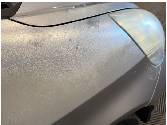
20: Wing osf Poor Previous Repair Paint Flake
