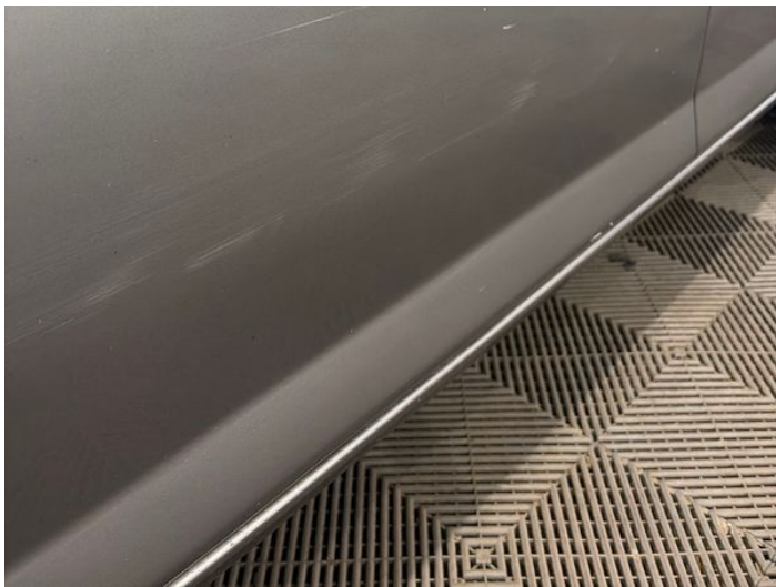
5: Door nsf Scratched Over 25mm Thru Paint
