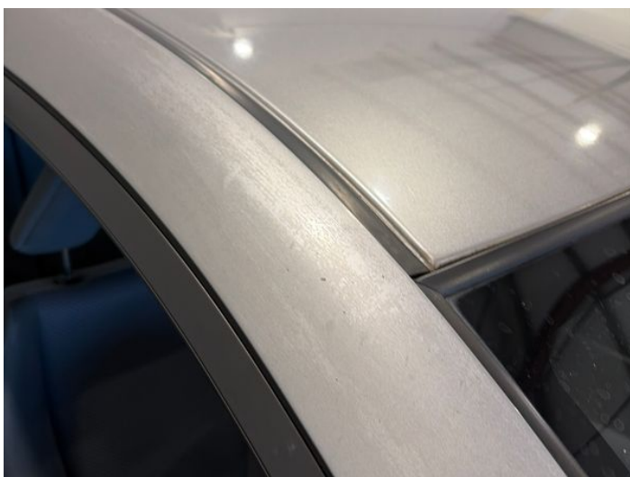
19: A Post os Poor Previous Repair Paint Flake
