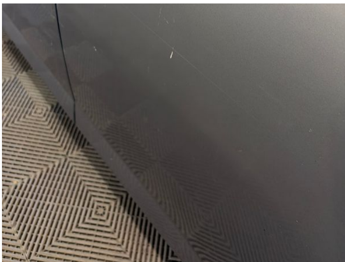
7: Door nsr Scratched Over 25mm Thru Paint
