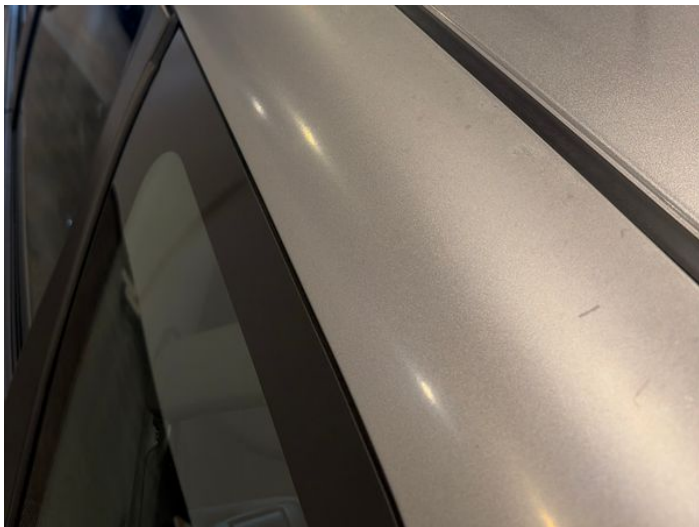
11: B Post ns Poor Previous Repair Poor Paint
