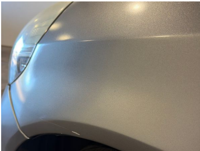
3: Wing nsf Poor Previous Repair Poor Paint
