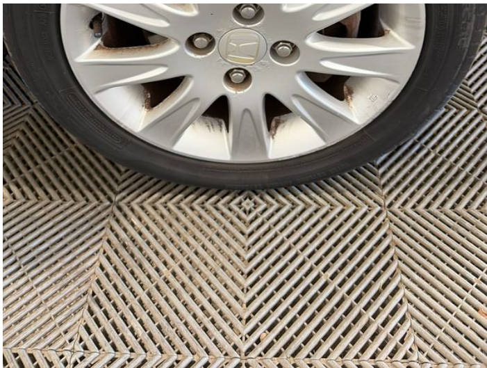
21: Wheel of Corroded Light
