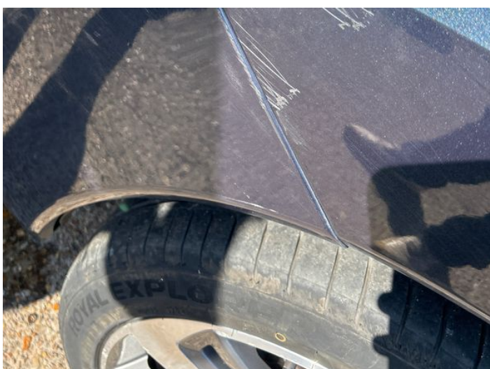
13: Wing nsf Scratched Over 25mm Thru Paint
