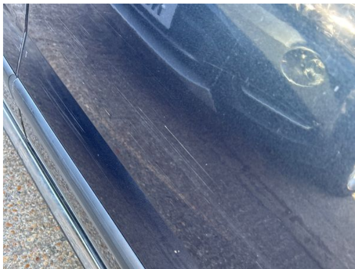
2: Door osf Scratched Over 25mm Thru Paint
