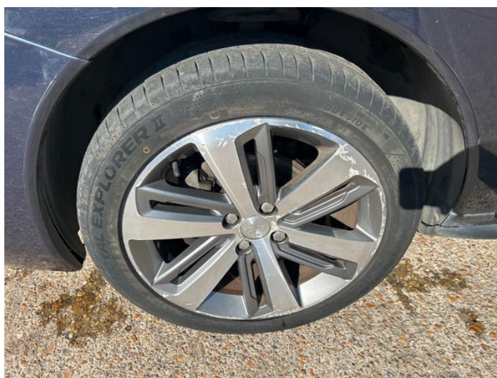
12: Wheel nsf Scratched Over 50mm
