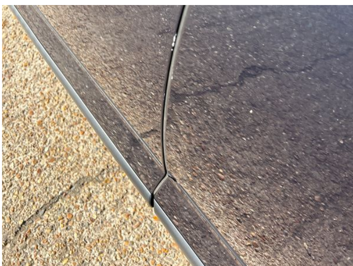
11: Door nsf Chipped Edge Chip
