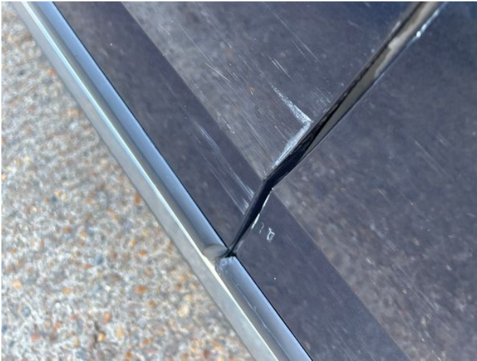
3: Door osr Scratched Over 25mm Thru Paint
