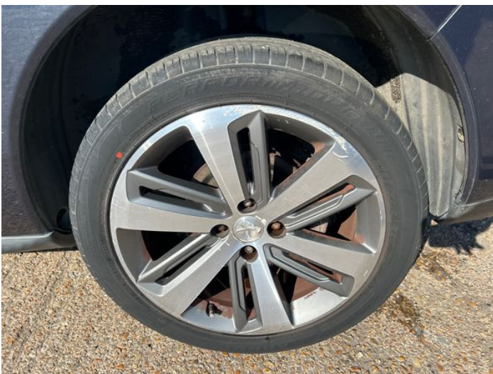
7: Wheel nsr Scratched Over 50mm
