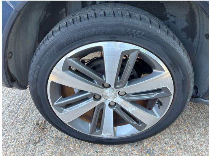
4: Wheel osr Corroded Light
