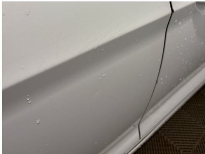
10: Door osr Scratched Over 25mm Thru Paint
