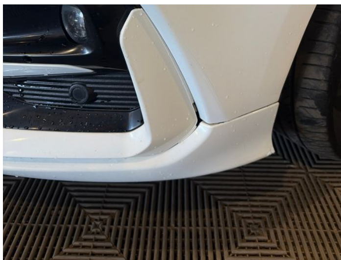
2: Bumper Front Dented With Paint Damage
