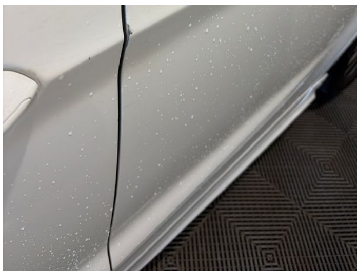
6: Door nsr Dented With Paint Damage
