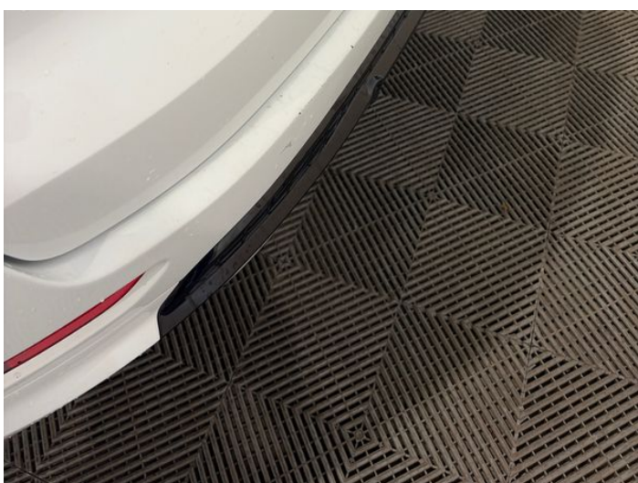
7: Bumper Rear Scratched 25 to 100mm Thru Paint
