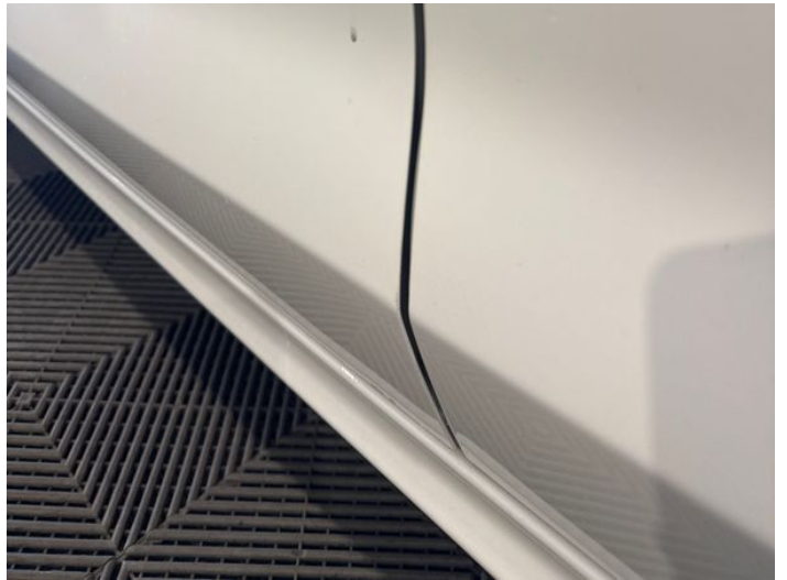
6: Door nsf Chipped Edge Chip
