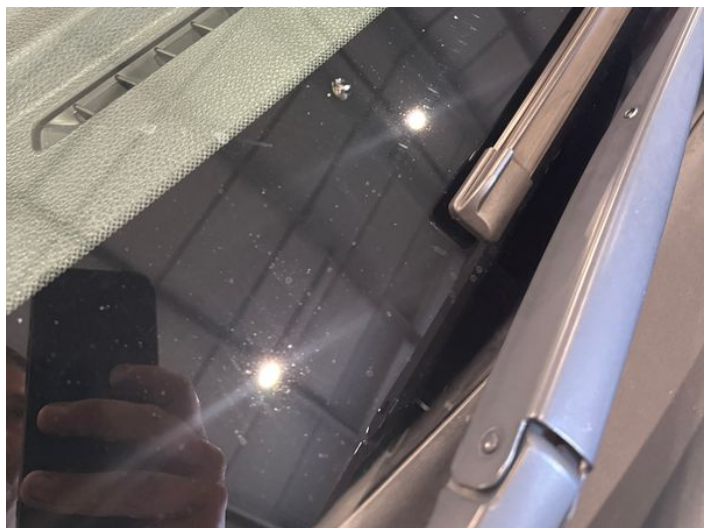
20: Screen Front Chipped Over 10mm
