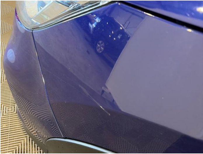
3: Wing nsf Scratched Over 25mm Thru Paint
