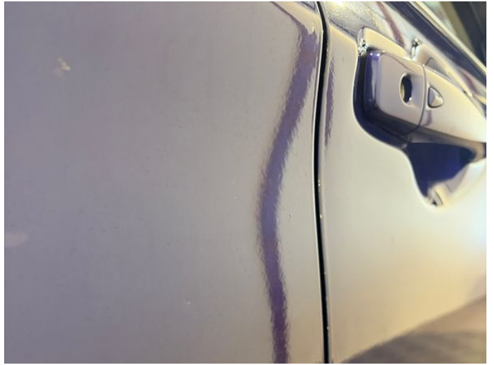
16: Door osr Dented Between 10mm + 30mm
