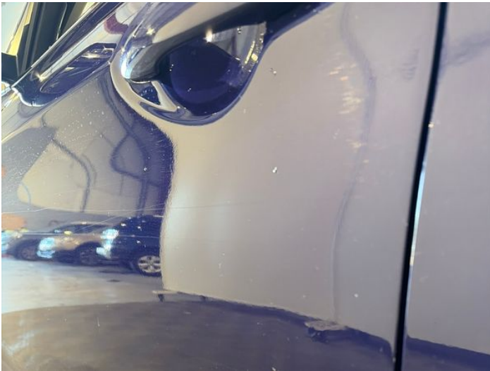
5: Door nsf Dented Over 30mm
