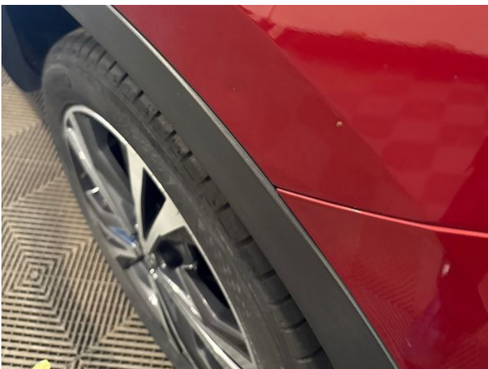
7: Qtr Panel nsr Dented Between 10mm + 30mm
