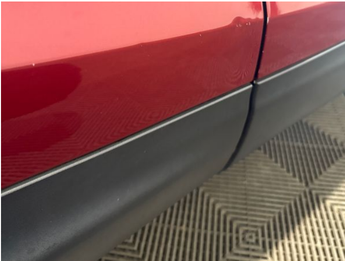
11: Door osr Dented Between 10mm + 30mm
