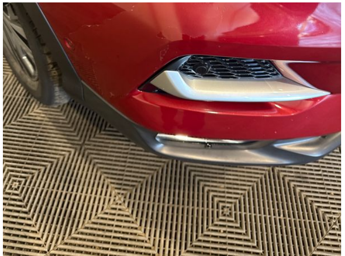
2: Bumper Front Poor Previous Repair Paint Flake
