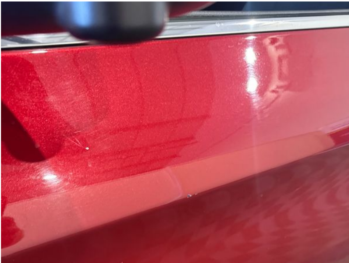
5: Door nsf Chipped 1 To 5
