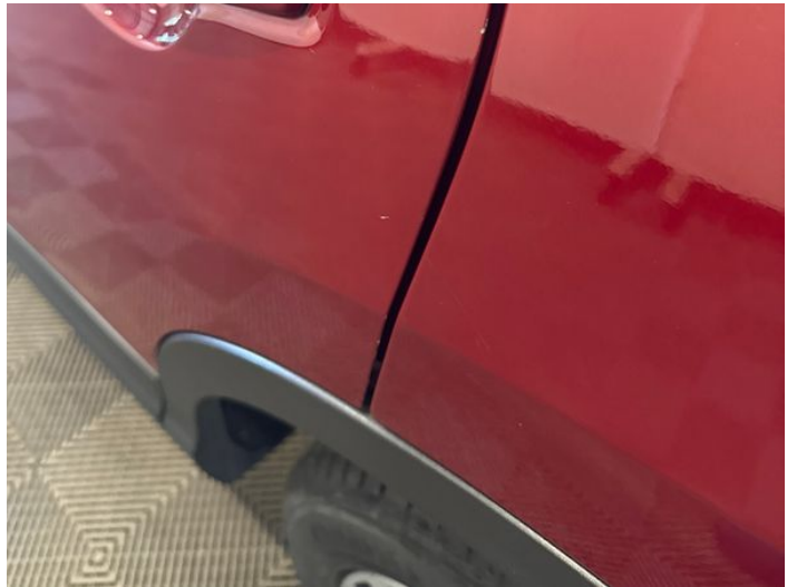
6: Door nsr Chipped Edge Chip
