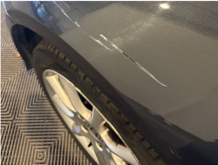
5: Wing nsf Scratched Over 25mm Thru Paint
