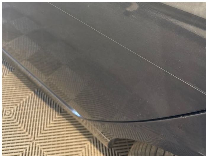
10: Door nsr Scratched Over 25mm Thru Paint
