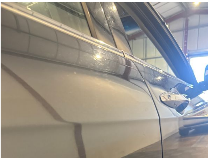
19: Door osr Dented Over 2 UpTo 10mm
