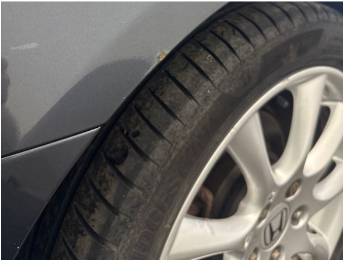
17: Qtr Panel osr Rusted Over 5mm
