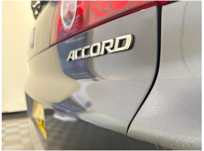
16: Tailgate Poor Previous Repair Rippled UpTo 30%
