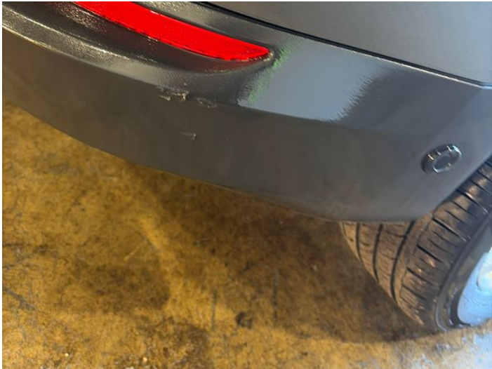
28: Bumper Rear Moulding Scuffed (Unpainted) UpTo 100mm
