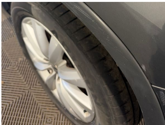
12: Qtr Panel Moulding ns Scuffed (Unpainted) Over 100mm
