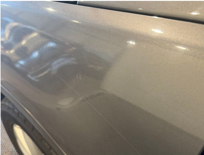
5: Wing nsf Scratched Over 25mm Thru Paint
