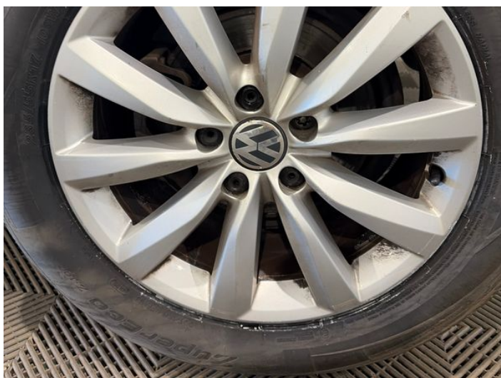
13: Wheel nsr Scratched Over 50mm
