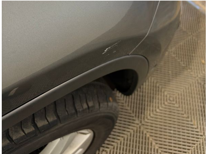
22: Wing osf Scratched Over 25mm Thru Paint
