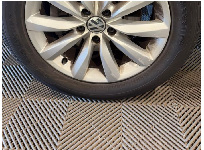
4: Wheel nsf Scratched Over 50mm
