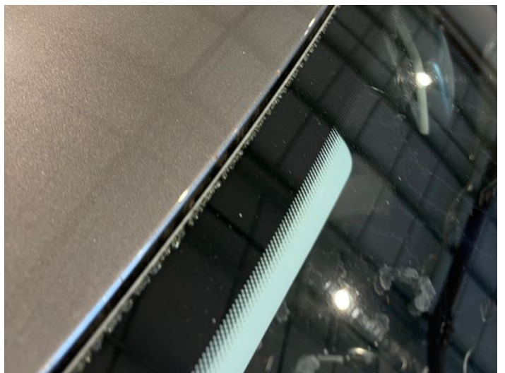
26: Roof Chipped Edge Chip
