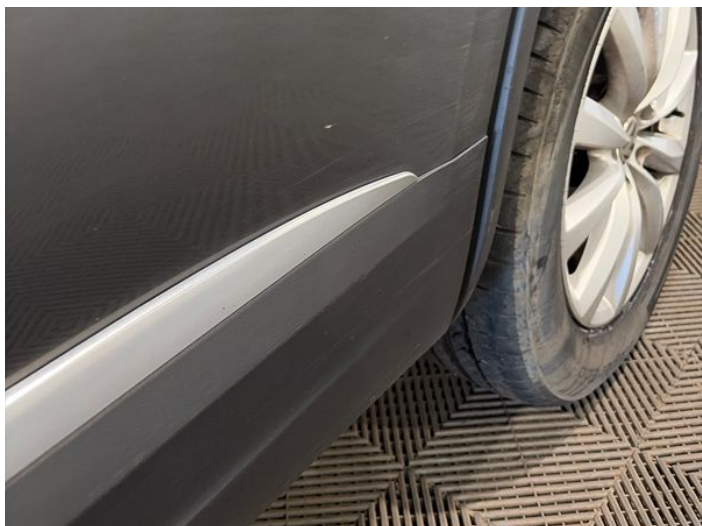
9: Door nsr Scratched Over 25mm Thru Paint
