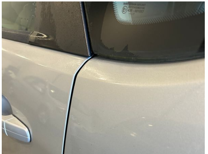
6: Qtr Panel nsr Dented Between 10mm + 30mm
