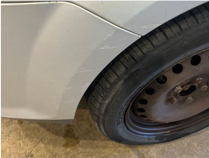
10: Bumper Front Scratched Over 100mm Thru Paint
