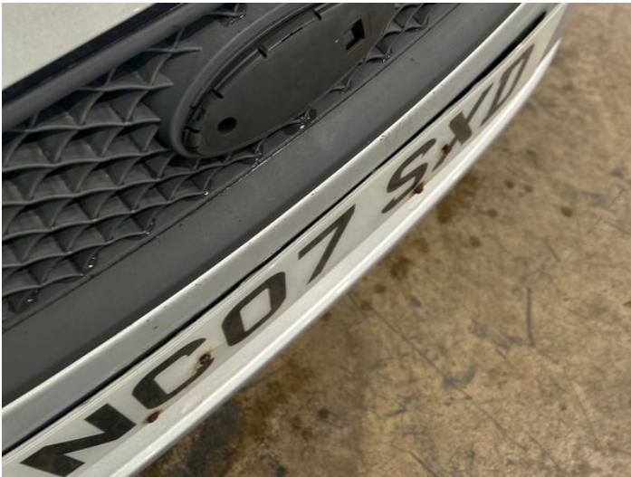
11: Badgedecal Front Missing Replace
