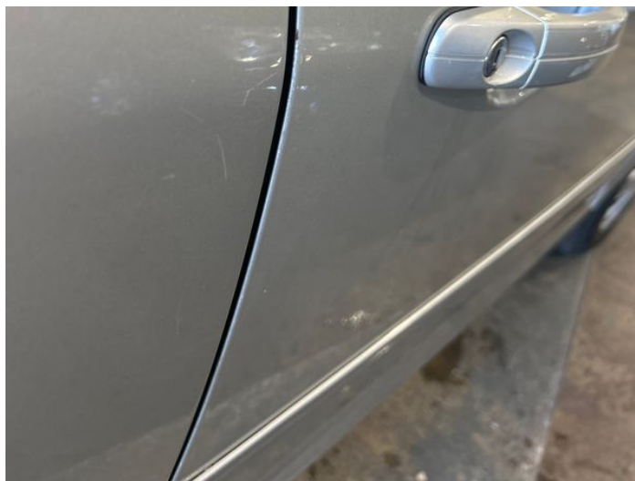
2: Door osf Chipped Edge Chip
