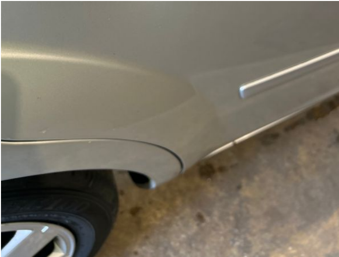
3: Door osr Dented With Paint Damage
