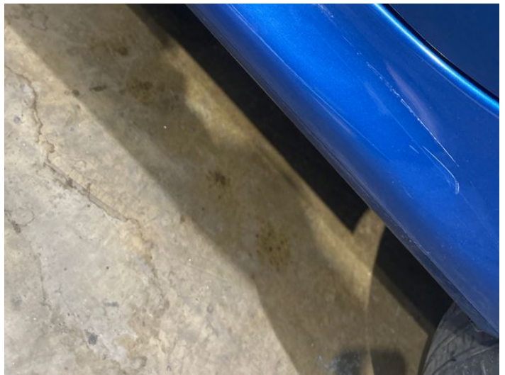
12: Sill ns Scratched Over 25mm Thru Paint
