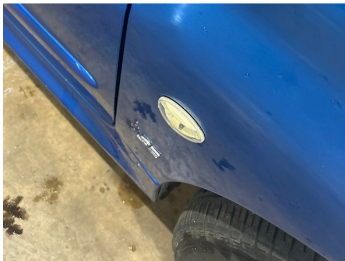
2: Wing osf Dented Over 30mm
