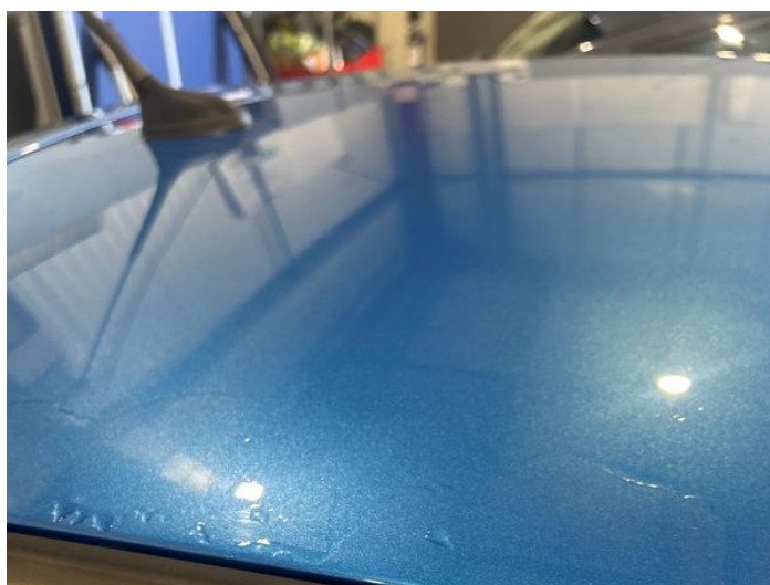
18: C Post os Poor Previous Repair Paint Flake
