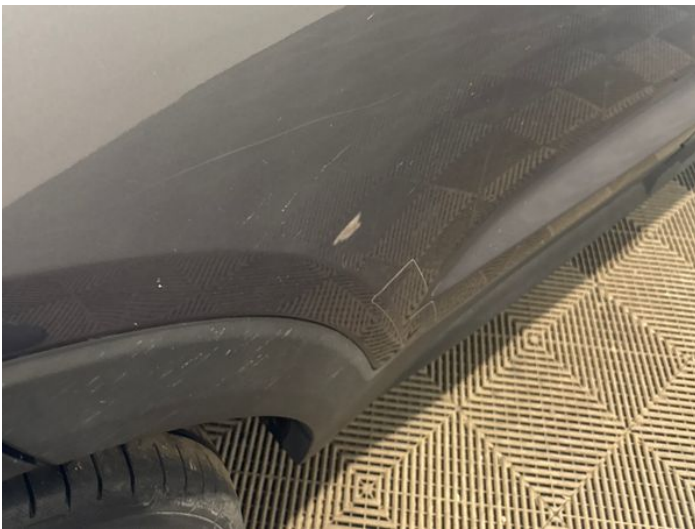
11: Door osr Scratched Over 25mm Thru Paint
