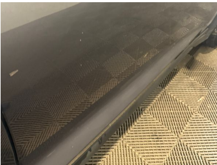
13: Door osf Scratched Over 25mm Thru Paint
