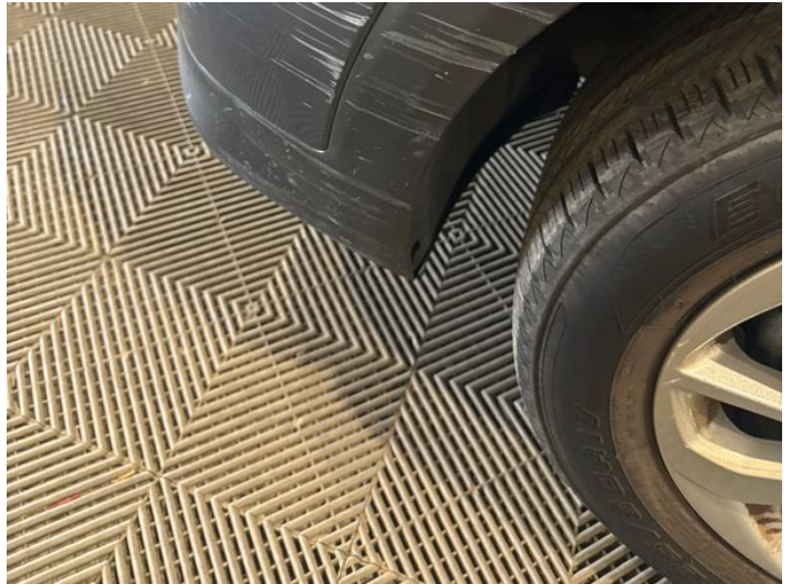
4: Bumper Front Moulding Scuffed (Unpainted) Over 100mm
