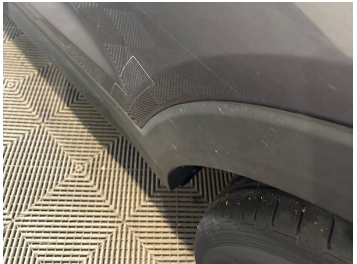
6: Door nsr Scratched Over 25mm Thru Paint
